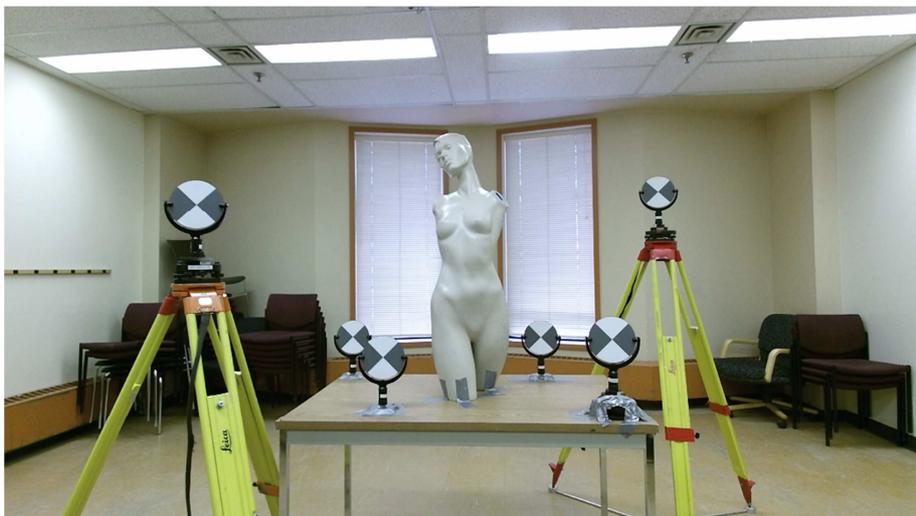
Figure 4: Setup of mannequin and retro-reflective targets for registration in static environment
