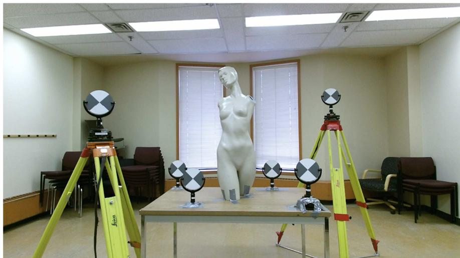
Figure 4: Setup of mannequin and retro-reflective targets for registration in static environment
