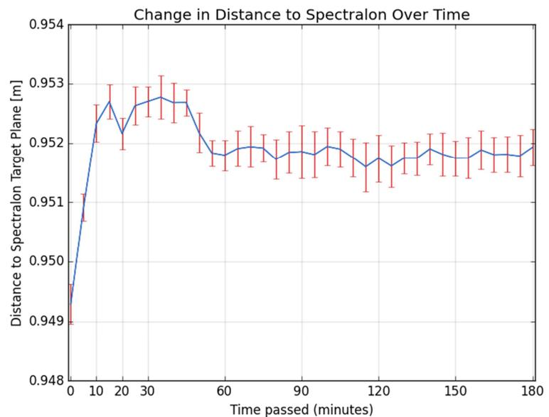
The reason why the Kinect 2.0 performs as it does with respect to warm-up time may potentially be attributed to the fans mounted to the exterior as part of the cooling system of the Kinect 2.0 sensor. Given that the Kinect 2.0 was originally designed for controlling home entertainment systems, this quick stabilization and long-term consistency could likely have been a part of its engineering design.
