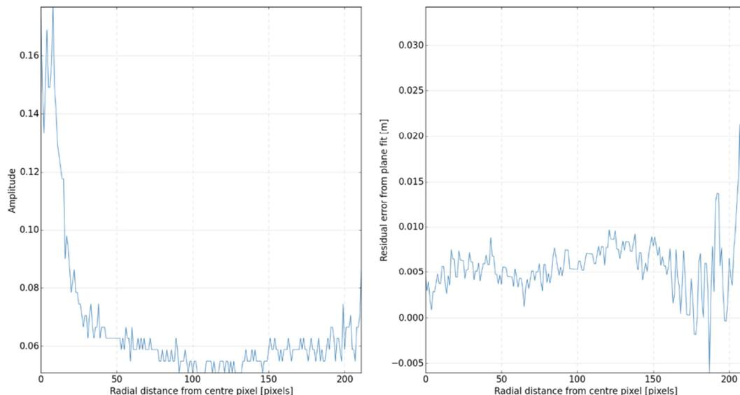
Figure 7: Diagonal cross-section of a) an amplitude image (left); and b) corresponding range residuals (right)
