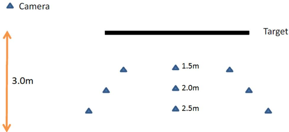
Figure 3: Plan view of camera setup locations. At each setup four sets of images are captured (36 in total).
