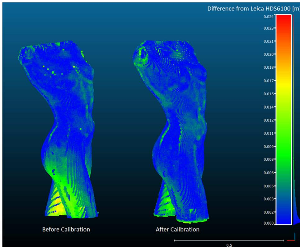
Figure 8: Results of torso reconstruction before calibration (left) and after calibration (right) of Kinect 2.0 data in reference to Leica HDS6100 laser scanner.
