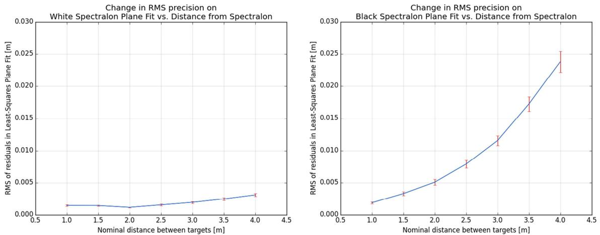
Figure 6: a) Change in RMS precision of plane fit as a function of distance using white Spectralon (left); b) Change in RMS of plane fit as a function of distance using black Spectralon (right)
