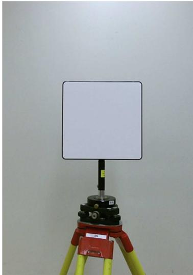
Figure 1: Spectralon planar target with 99% albedo (reflectivity)
