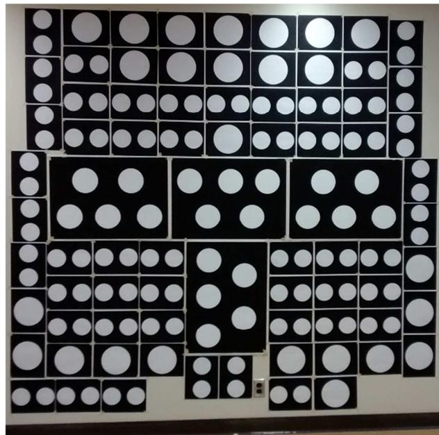
Figure 2: Target field used for self-calibrating bundle adjustment
