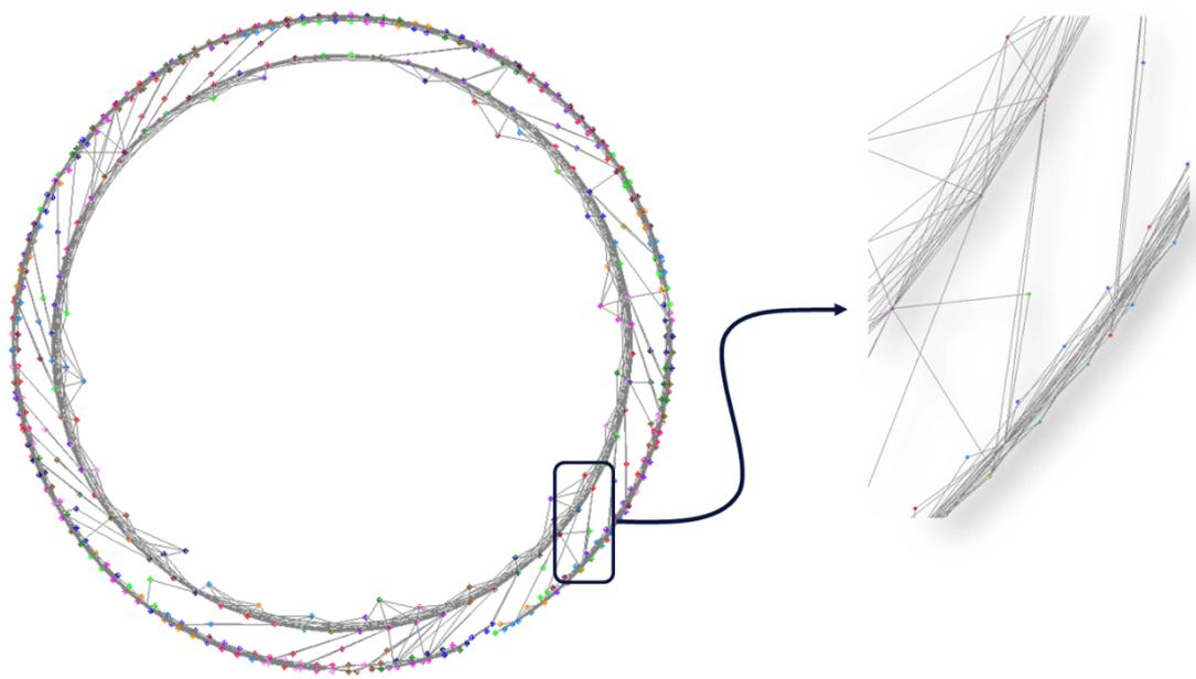
Figure 3 This image shows the EX2 survey network. It is one of the ESRF networks comprising several hundred points measured by highly redundant 3D observations - horizontal and vertical angles, and slope distances. It forms the backbone for the individual beamline networks. Grey lines show laser tracker observations.
