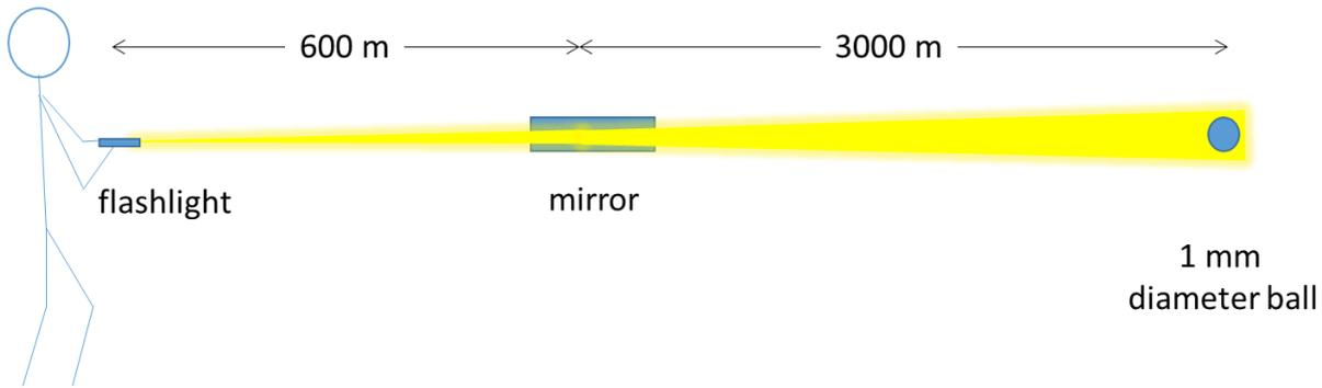
*Figure 1 To appreciate this alignment challenge, consider shining a 20 mm diameter flashlight beam onto a mirror located 600 m away from where you are with the flashlight, and aiming so that the reflected beam illuminates a 1 mm diameter ball located at a distance just over 3 km from the mirror.*
