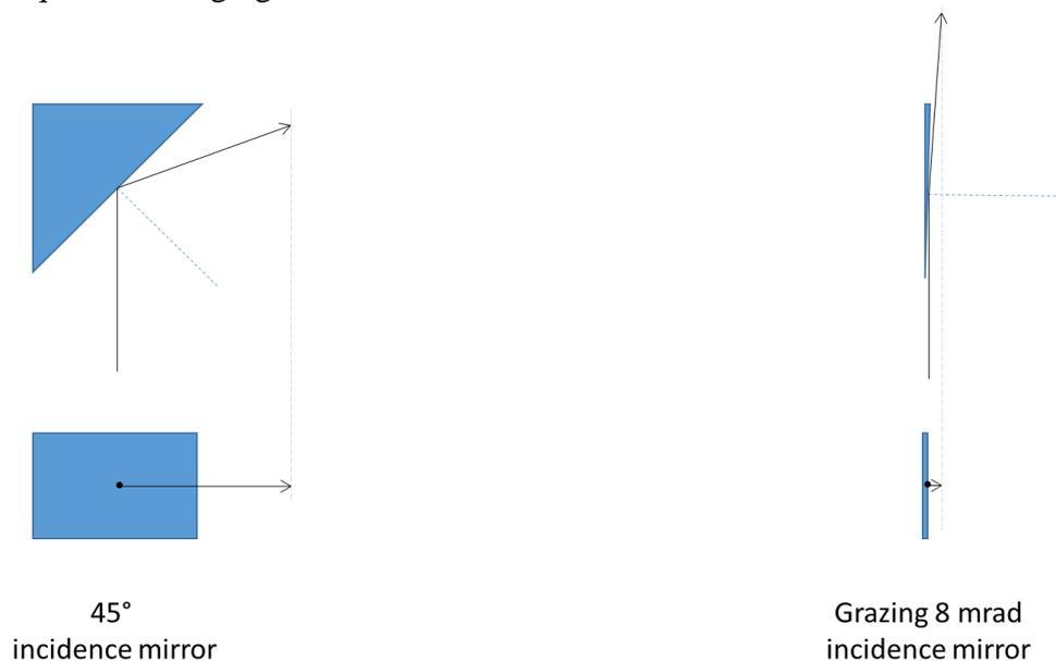
*Figure 5 On the left hand side a mirror rotated 45° to an incoming beam of light. On the right a mirror rotated at a grazing angle of 8 mrad to an incoming beam of light.*
