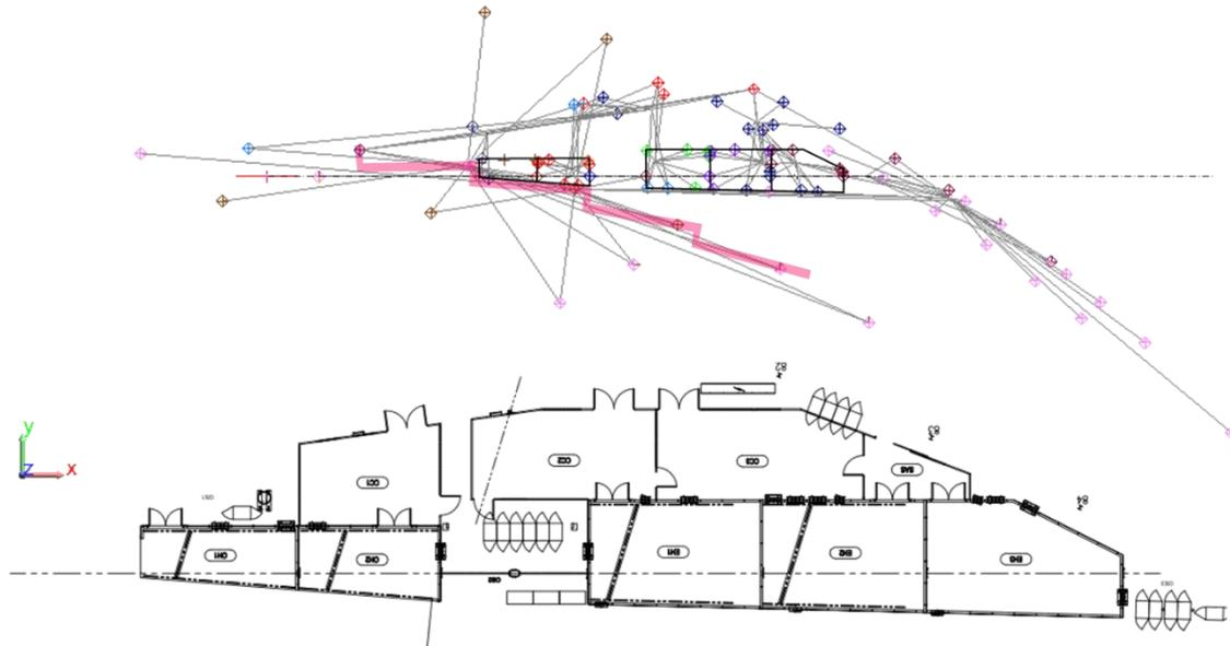
Figure 4 Typical beamline reference point network. The top part of the figure shows the network with the outline of the beamline hutch walls. The experimental hutch layout on the same beamline is shown in detail in the lower part of the figure. The photon beamline axis is shown as a dashed line in the top and bottom parts of the figure. Grey lines represent laser tracker observations made from the main ESRF network to the experimental hutch networks.
