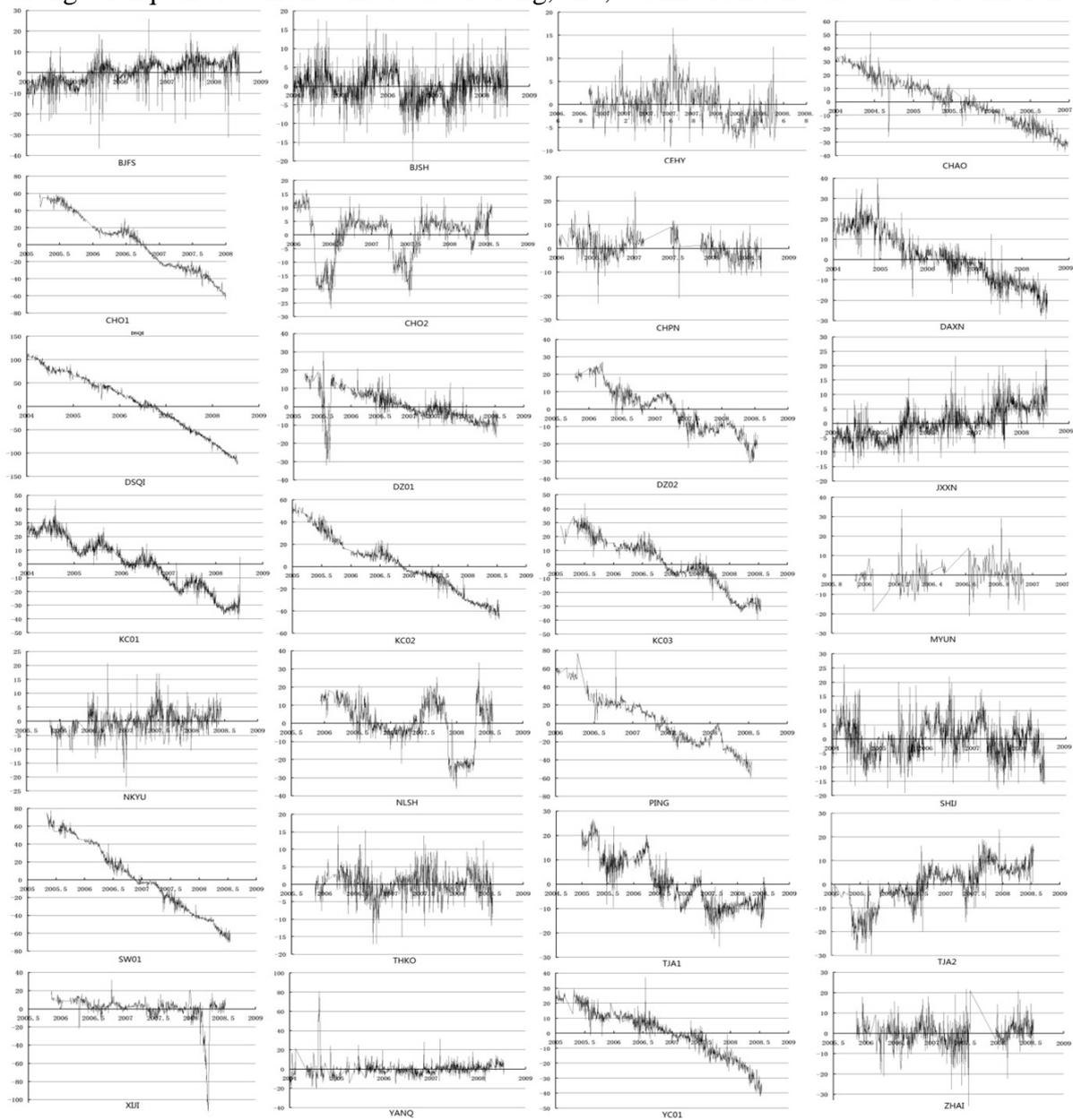
Figure 2 Vertical component time series of some GNSS observations
