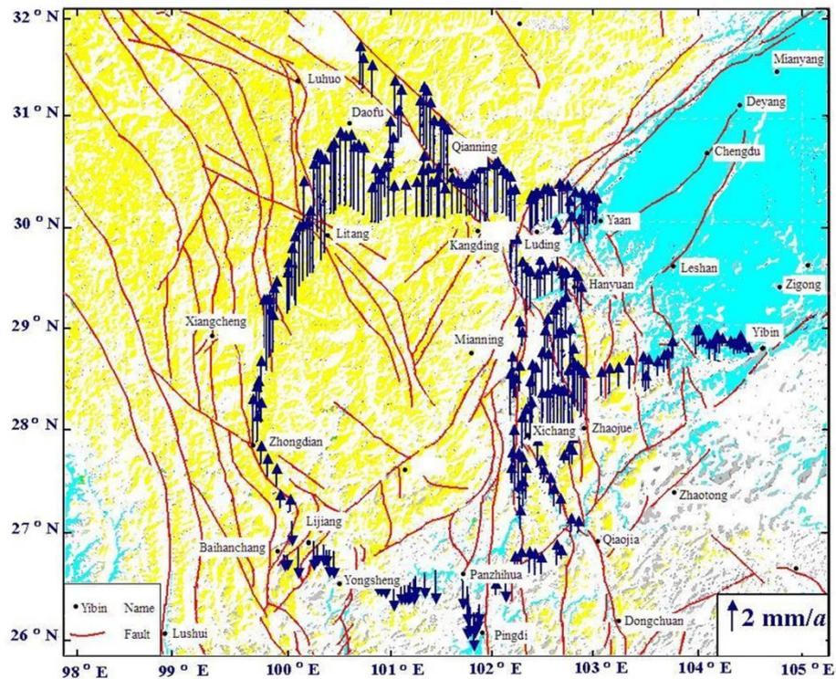
Figure 6 Vertical displacement rates of leveling bench marks in sichuan-yunnan region(with a reference mark of Yibin, according to Wang Q L)
