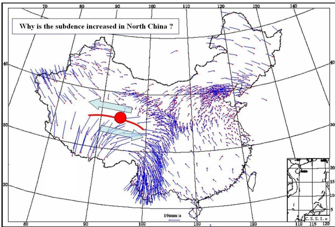
Figure 4 Sketch map of the left-lateral rupture of Ms8.1 Kunlun Mountain earthquake and horizontal deformation field of China Continent under regional no-net-rotation reference frame (Hu X K *et al*, 2007)
