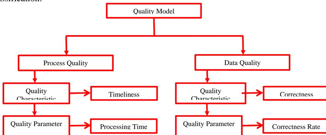
Figure 3: Structure of the quality model for the detection and classification cracks
