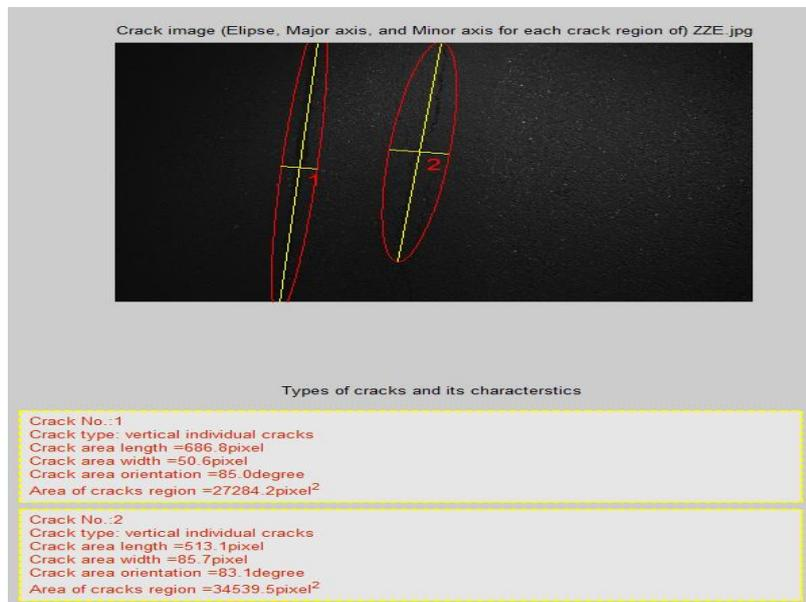
Figure 4: Detected and classified vertical individual cracks
