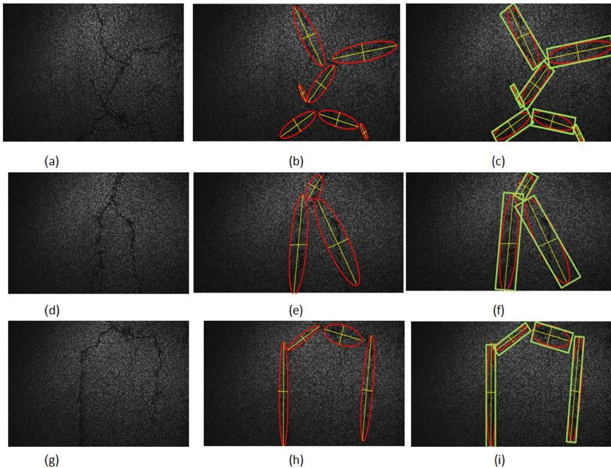
Figure 2: Behavior of the modified algorithm to count the number of block cracks branches within image; the first column represents the original images of block crack type; the second column represents the block crack shape after applying modified binary mask algorithm (AL-MISTARHI&SCHWIEGER 2015); the third column represents the block crack shape after moving rectangle binary mask over ellipses regions. The three lines show different examples of block crack types
