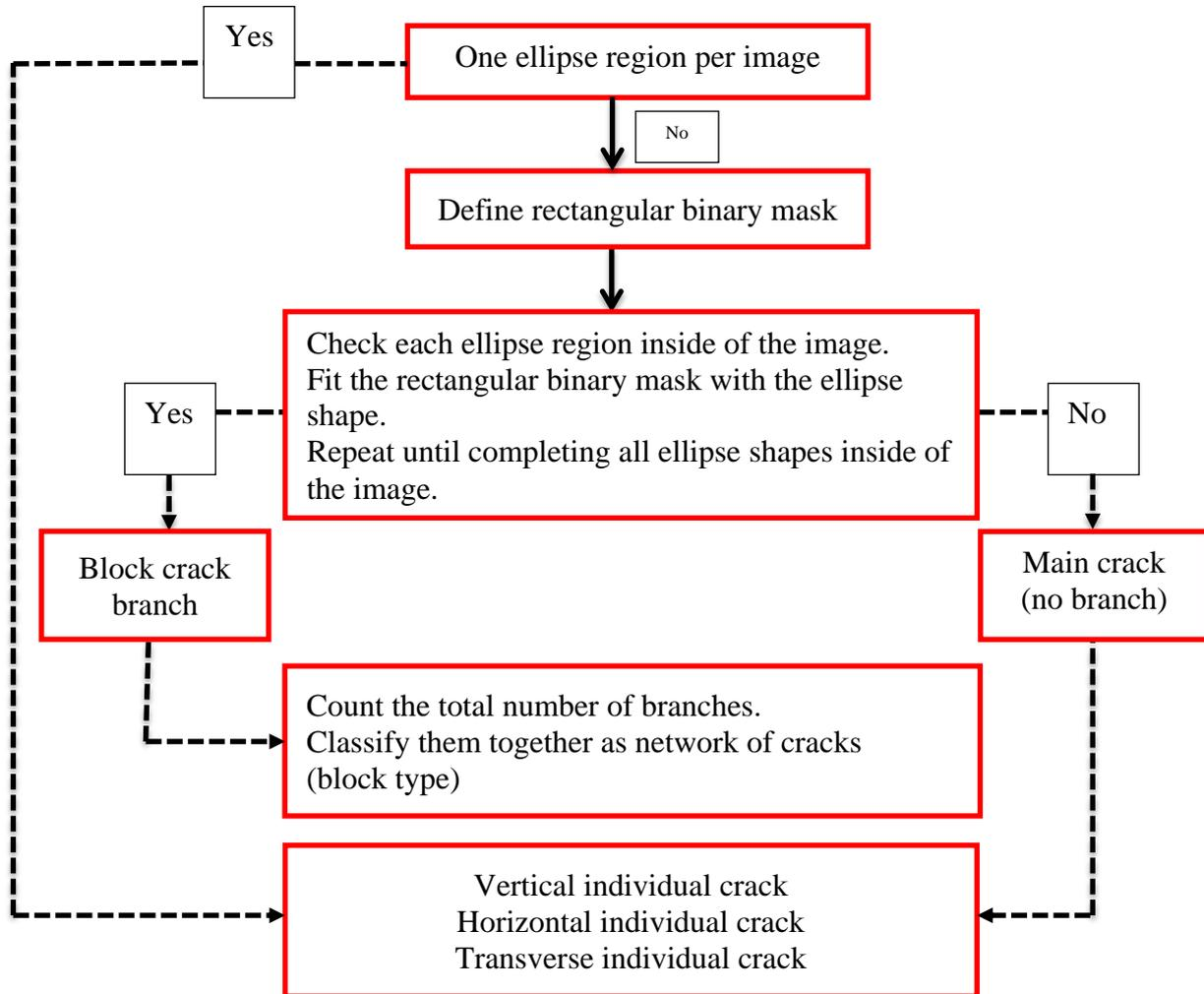
Figure 1 : Workflow for the modified algorithm to classify cracks into different types during detection stage
