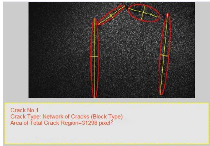
Figure 5: Detected and classified network of cracks (block type)
