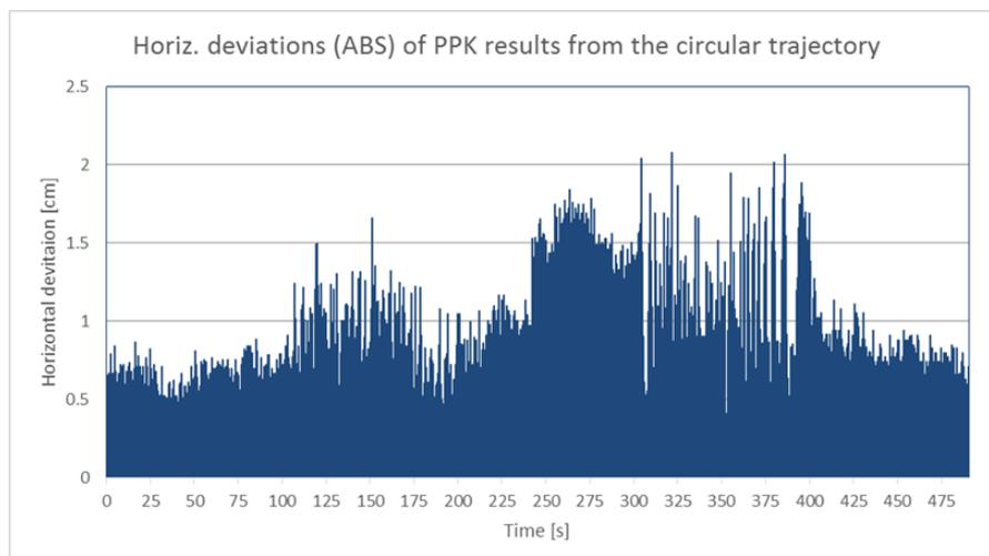
Figure 7. Horizontal deviations (absolute values) of PPK results from the theoretical circular trajectory.
