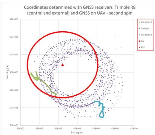
Figure 10. Points determined during the 1<sup>st</sup> spin.
