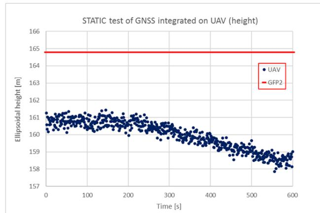
Figure 3. Results of STATIC test (height).
