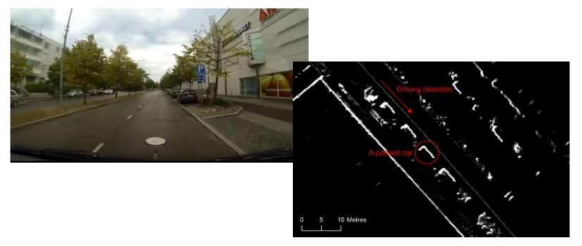
**Figure.** a) Part of the street Espoonlahdenkatu as recorded on the reference video during data acquisition Drive 1. b) Raster representation of the car-based laser scanner data. The pixel value of each  $0.3 \text{ m} \times 0.3 \text{ m}$  cell corresponds to the number of laser points inside the cell. Parked cars appear as L shaped clusters of bright pixels.
