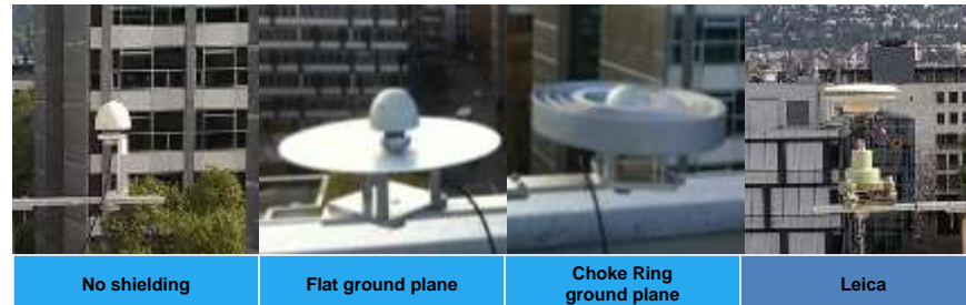
Four combinations of antenna-shieldings
