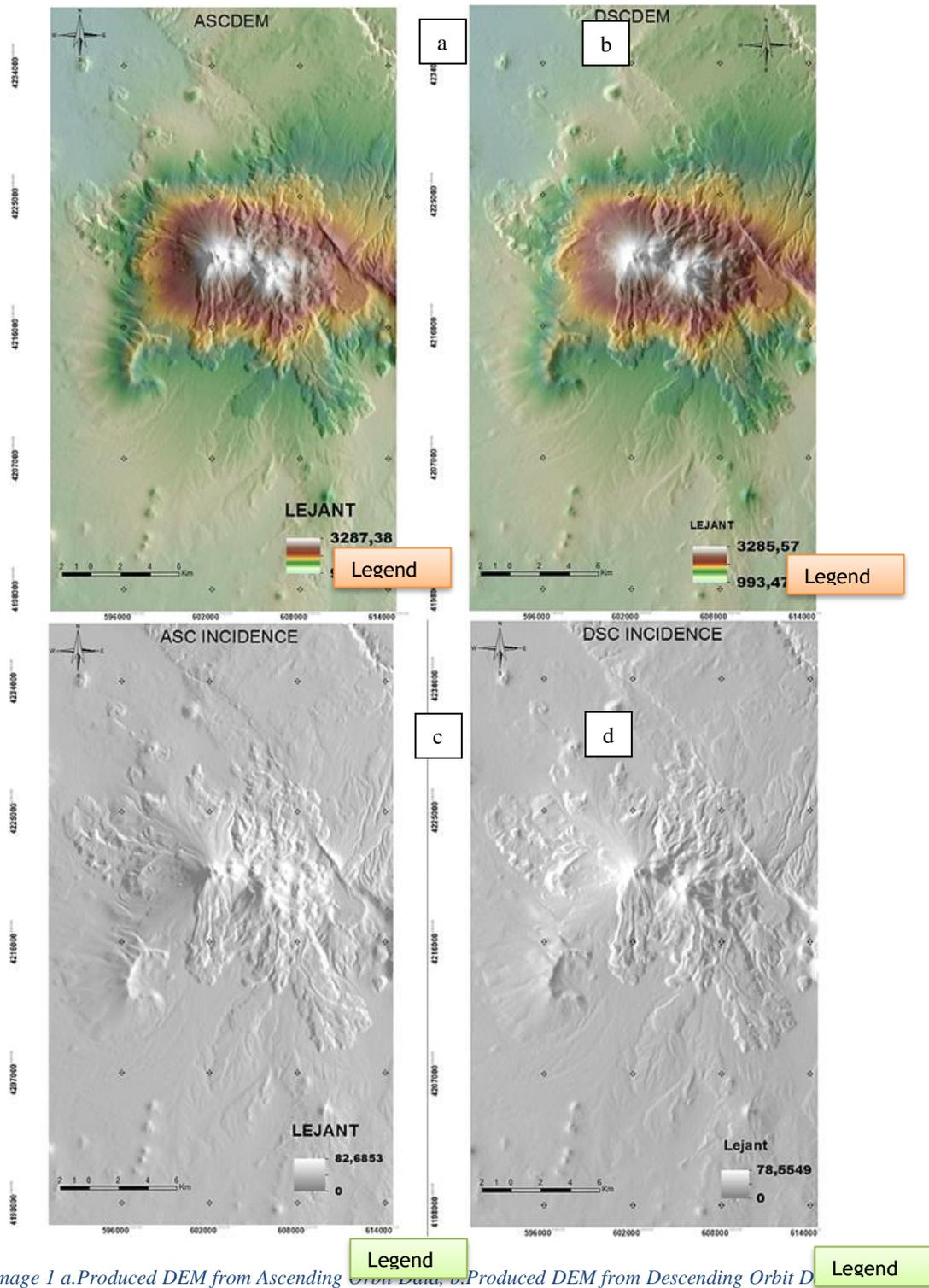
Image 1 a. Produced DEM from Ascending Orbit Data, b. Produced DEM from Descending Orbit Data, c. Incidence Angle of Ascending Orbit Data, d. Incidence Angle of Descending Orbit Data
