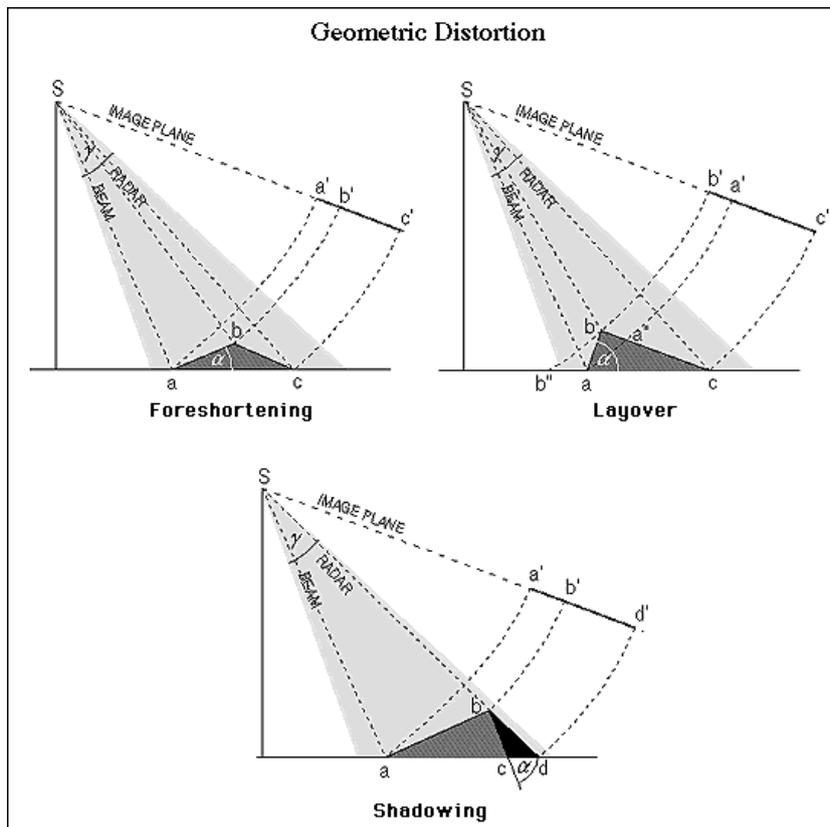
Image 6 Geometric Distortions of RADAR
