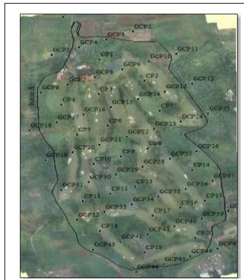
**Figure 2. GCP and ICP distribution plans**
