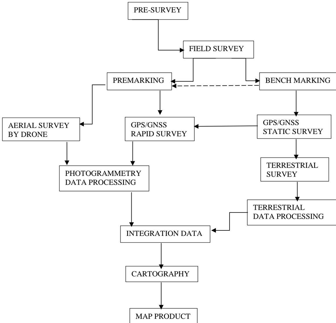
Figure 1. Methodology of Photogrammetry – UAV Method
