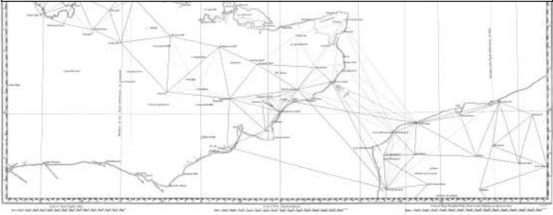
Figs. 9 & 10 Jesse Ramsden Great Theodolite for the UK Triangulation Survey and Map showing the triangles measured to determine the longitude variation between Greenwich and Paris Observatories.
