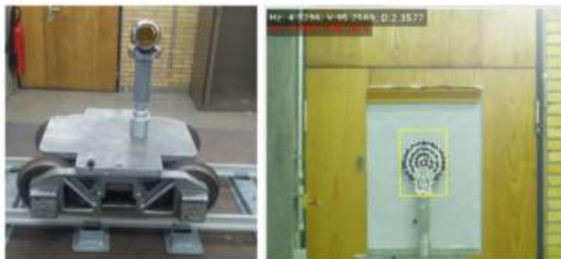
Figure 8. Moving trolley with laser tracker reflector (SMR) (left) and the target with feature points as identified by the IATS (right)
