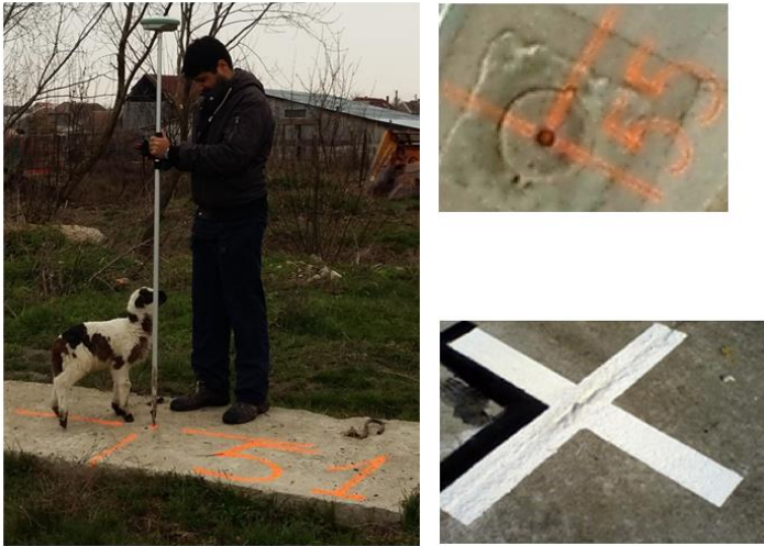
Figure 1.1.2 Pre-signaling the control points on the ground
