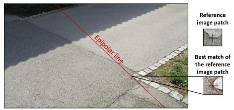
**Figure 4** The matching algorithm searches for the best match of the reference image patch along the epipolar line to find the corresponding points.
