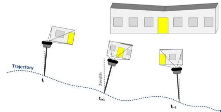
**Figure 1** Schematic illustration of the measurement workflow of the presented image-based surveying approach, where images are recorded at epochs  $(t_i, t_{i+1}, t_{i+2}, ...)$  while passing the scene of interest.
