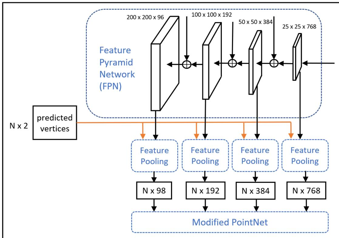
**Figure 2. Detailed structure of the improved feature pooling process.**
