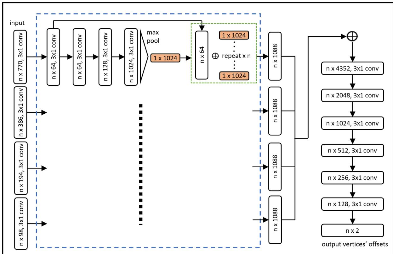
**Figure 3. The improved BRegNet which enables multi-scale feature vector inputs**
