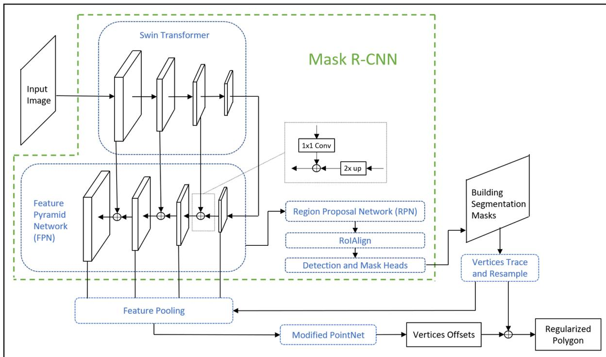
**Figure 1. Integration of the Feature Pyramid Network with PolygonCNN.**
