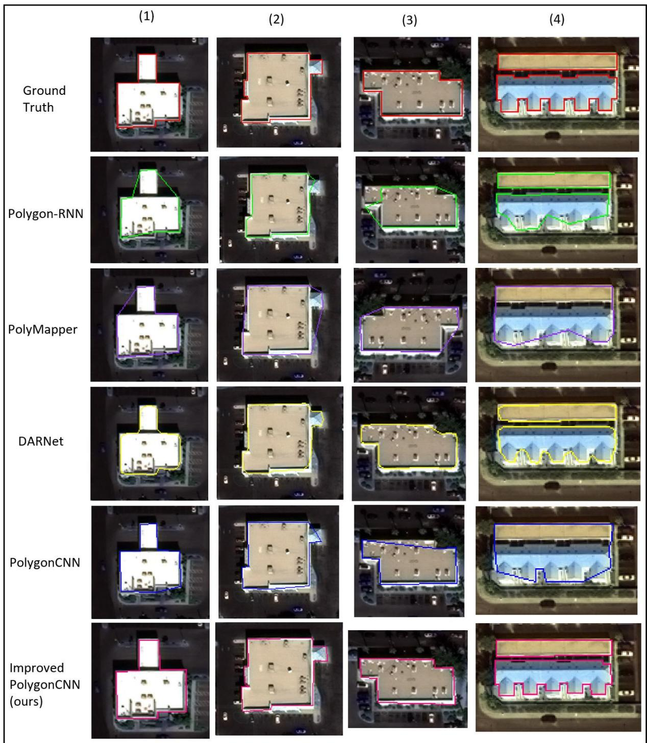
**Figure 4. Examples of building vectors generated by Polygon-RNN, PolyMapper, DARNet, PolygonCNN, and our improved PolygonCNN.**
