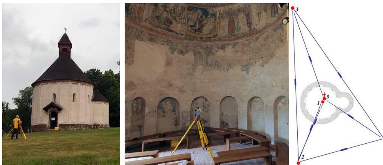
Fig. 10. The Selo rotunda outside, inside and the sketch of control point network
