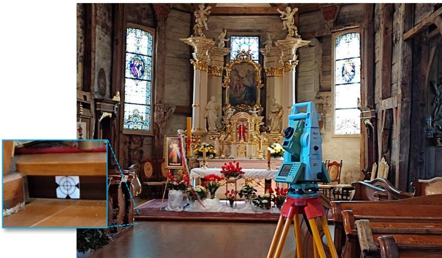
Fig.5. Leica TCRP 1201+ total station in the station in the center of the nave; on the left side, a reflective foil target – one of the points of reference.
