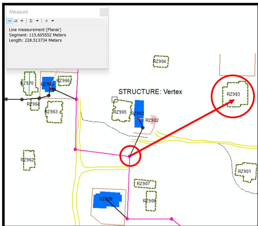
Figure 6: Estimating resources for connecting a new customer
