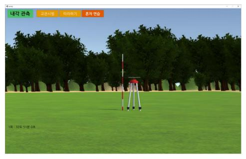
3. After moving to the left pole using a gamepad or keyboard, press the A button on gamepad or ctrl key on keyboard to take the first point. The angle between the first pole (Figure 2) and the second pole (Figure 3) is calculated and shown in the lower left.
