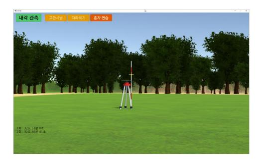
4. After moving to the left pole using a gamepad or keyboard, press the A button on gamepad or ctrl key on the keyboard to take the second point. Then, the angle between the picture 3 above and the second point taken this time is shown in the lower left corner.
