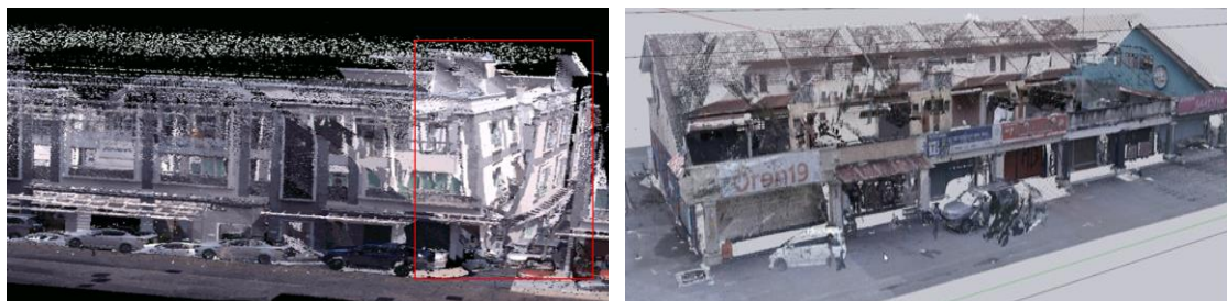
Figure 8: (L): Tilted Point Clouds Due to Sharp Turn Vehicle; (R): Incomplete Building Side Views
