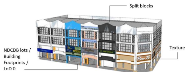
Figure 4: A 3D Model of a Shop House Block Segmented According to NDCDB Lots
