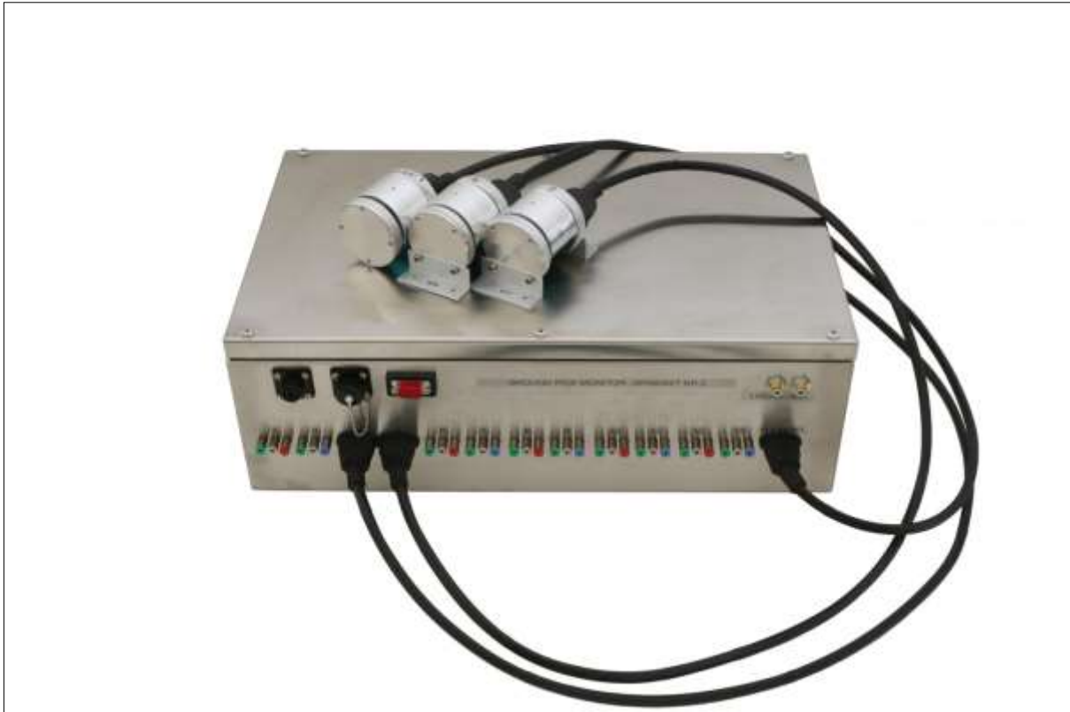
Fig. 3): GRIMONIT central unit with two measuring probes and the zero sample connected.
