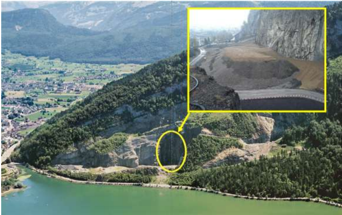
Fig. 4): Zingel quarry. The marked part of the first excavation was to be backfilled with waste slag, while siliceous limestone is still being mined in the rear part.
