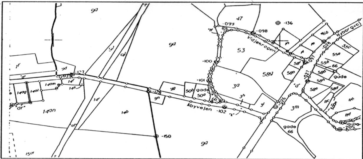
**Figure 6.** The digital cadastral map from 1993 shows the same area as figure 5, but the map is now linked to the national grid as a “frame map” showing only the current cadastral situation. The boundary points, shown by circles, are established in the map using control points and cadastral measurements. The digital cadastral map is thus tailored for integrated land management (Courtesy of the National Survey and Cadastre, Denmark).
