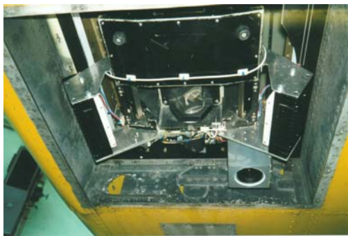
Fig. 4. Thermal scanner in Cessna 402
