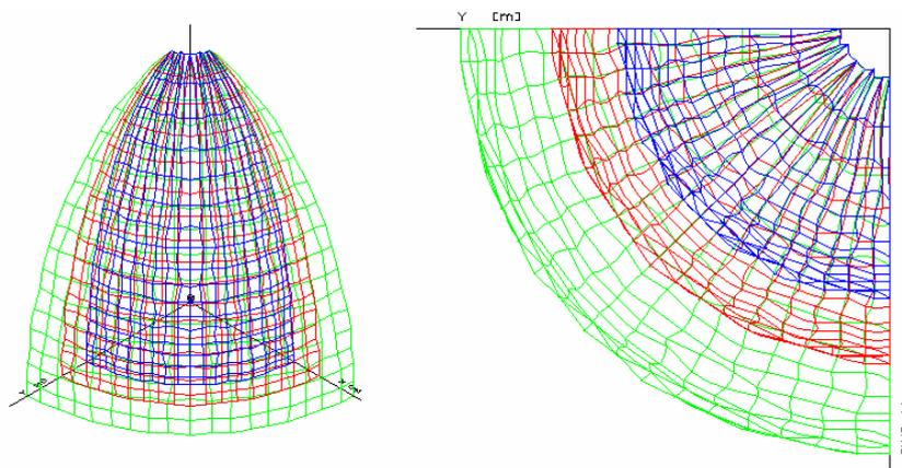
**Fig.3:** Surfaces with the same uncertainty in point position – Microstation SE software
