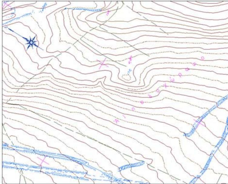
**Fig 2:** DTM derived from classical measurements
