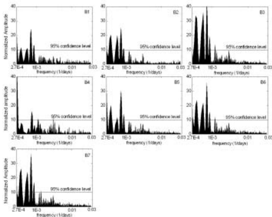
Figure 5: Spectra of the residuals of the displacements for all control stations of the Mandria landslide computed using the “Normperiod Code”, based on the Lomb periodogram. Statistically significant peaks (above the 95% confidence level, represented by a straight solid line), common in the spectra of the displacements of all control stations, are also shown and listed in Table 3.
