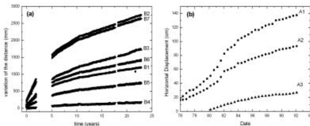
Figure 3: Distance changes versus time of seven (B1 to B7) control stations of the Mandria landslide (a) and of 3 control stations (A1, A2, A3) of the Alexis landslide (b), respectively, from stations in stable ground.
