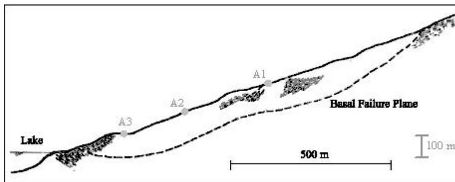
Figure 2: Cross section of the Alexis slide. The basal failure plane and the position of control points A1 – A3 are shown. For location see Fig. 1.
