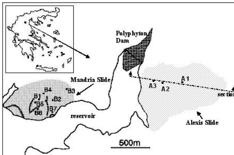
Figure 1: Location map of the Mandria and the Alexis landslides in the reservoir formed by the construction of the Polyphyton Dam. Control stations B1 – B7 and ground cracks (thin lines with ticks) of the Mandria landslide are also shown.
