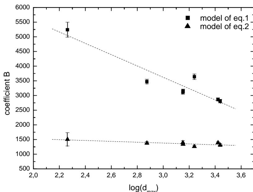
Figure 4: Plot of coefficients  $B_j$  of eq. (1) and eq. (2) versus  $\log(d_{max})$  for each control station  $j$  of the Mandria landslide. The dashed lines indicate the best fitting lines for the coefficients  $B_j$  of the models based on equations (1) and (2), respectively. The 95% confidence level bounds for coefficients  $B_j$  are also shown
