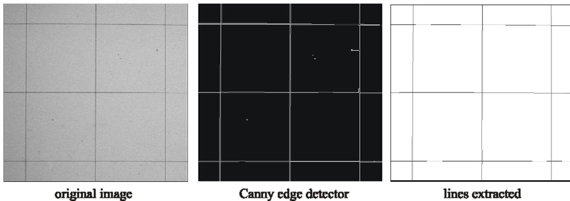
Figure 2: Identification of the grid lines
