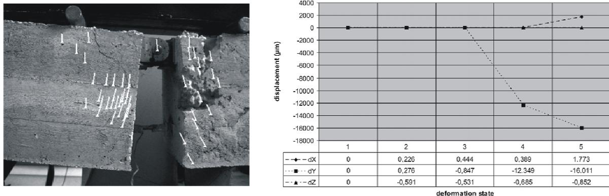
Figure 5: Deformation vectors and displacements
