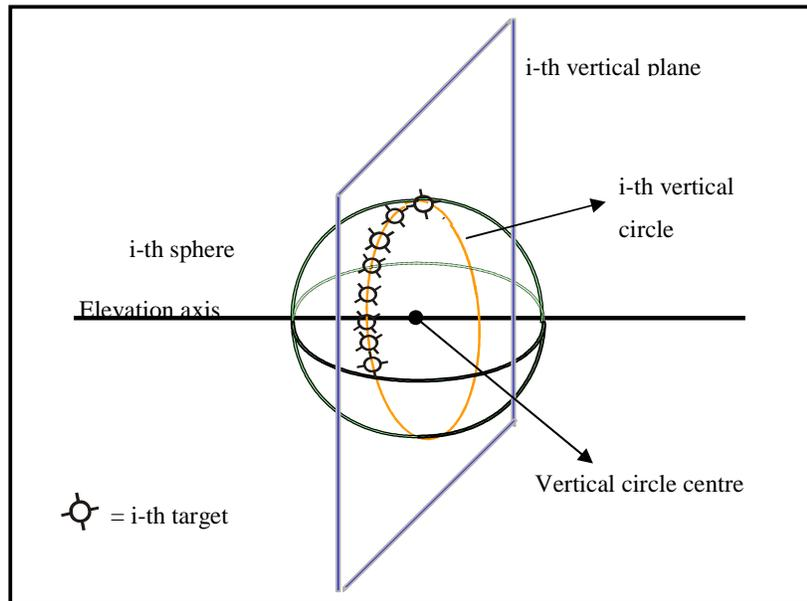
Figure 2: - Rotation in elevation of target *i-th*: definition of the elevation axis
