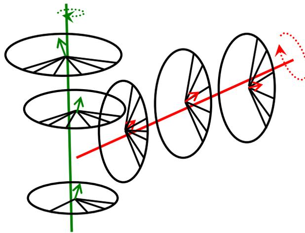
Figure 3: - targets' rotations around the elevation (red) and azimuth (green) axes; circles' centres, planes directions (arrows) and radius are shown.
