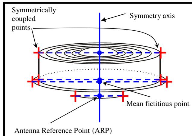
Figure 4: GPS antenna surveying scheme: the position of the ARP is indirectly recovered performing triangulation on symmetrical points identified on the edge of the antenna and applying geometric conditions on fictitious points.
