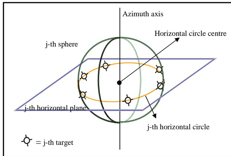
Figure 1: Azimuth rotation, horizontal circle centre, sphere and plane
