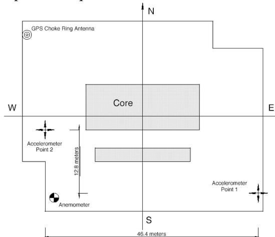
Figure 1 - Latitude Tower in the Sydney CBD. Figure 2- Plan view of Latitude Tower with major axes and orientation.
