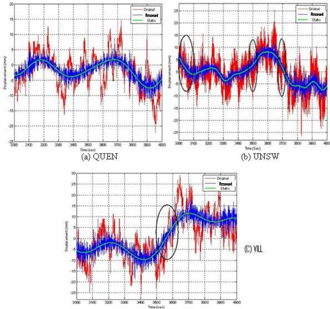
Figure 8 - Static displacement in x direction measured by GPS with different baseline lengths.
