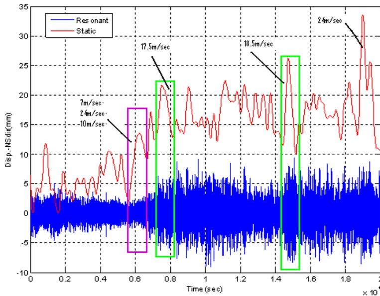
Figure 5 - GPS static & resonant displacements time series vs wind speed information.
