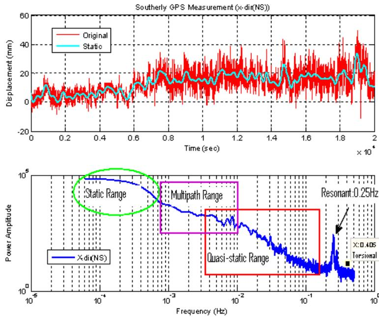
Figure 4 - GPS displacement time series in  $2 \times 10^4$  seconds and its spectrum.
