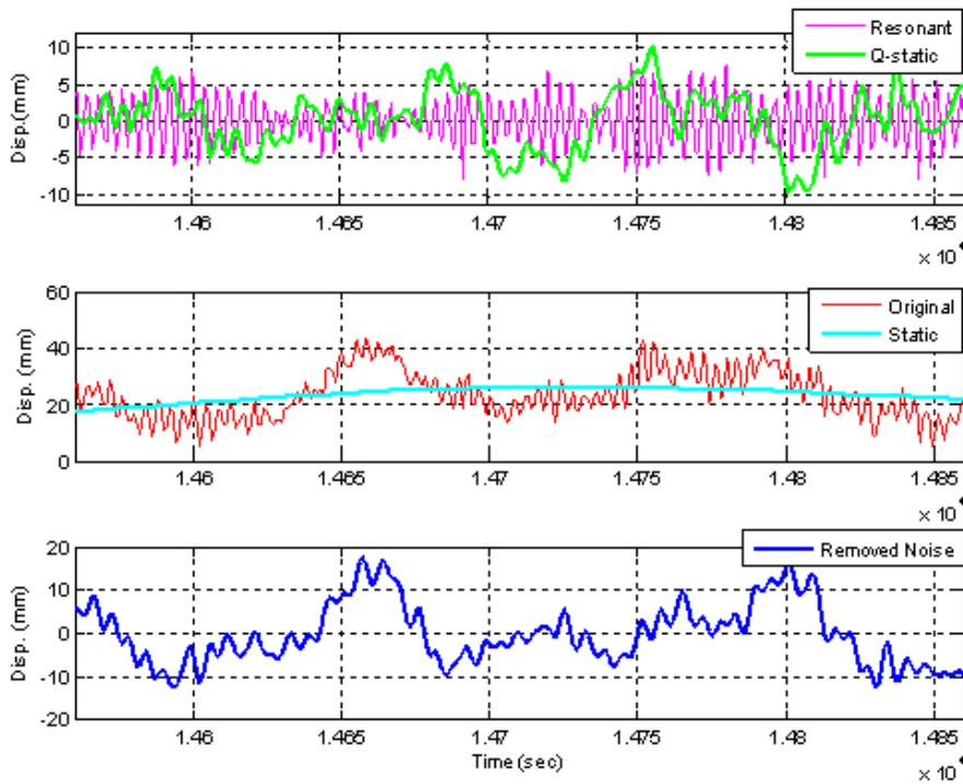
Figure 6 - The results of processing GPS measured components.
