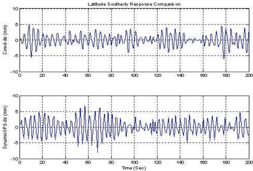
Figure 7 - Comparison between GPS-measured and accelerometer-derived resonant displacement.
