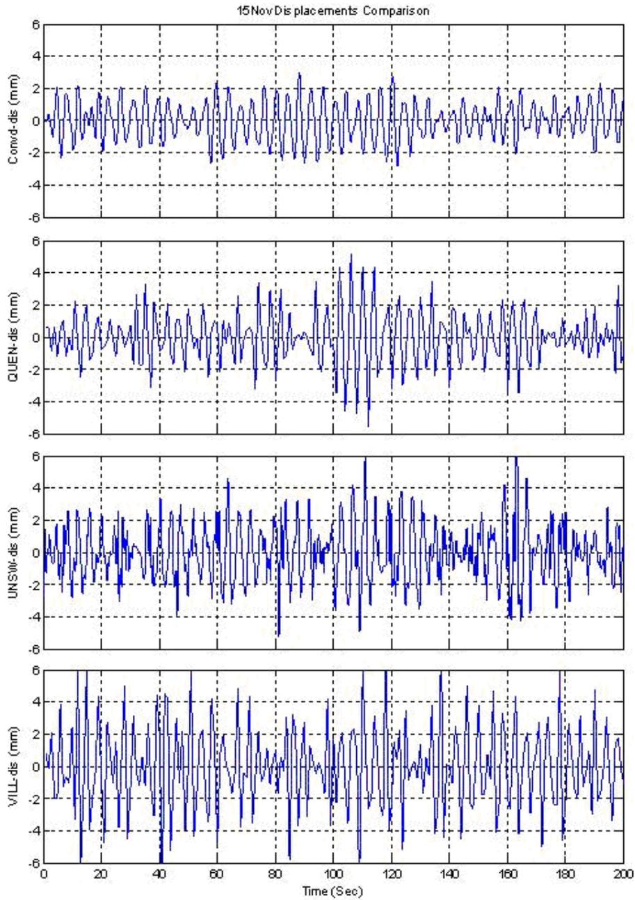
Figure 9 - Resonant displacement comparison - GPS with different baseline lengths vs accelerometer-derived values.
