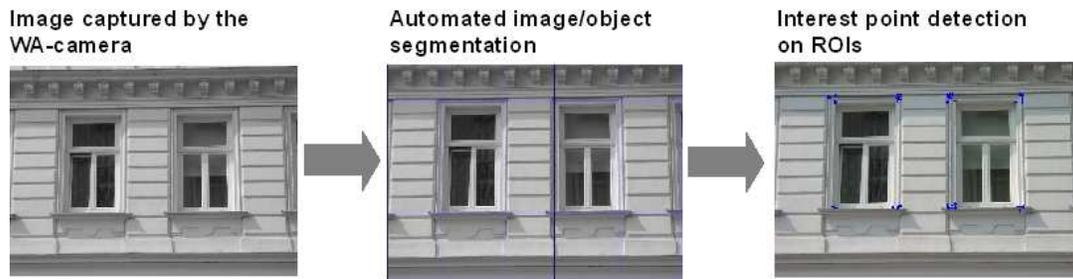
Figure 4 - Processing sequence of image point detection: An overview image is captured by the WA-camera. In a second step image/object segmentation is done. IPs are detected in the images captured by the internal IATS camera (overlaid to the WA-image).
