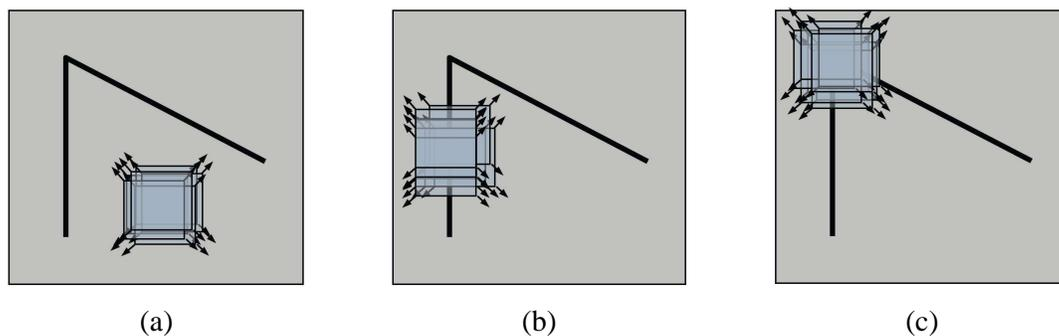
Figure 3 - Basic idea of an interest operator (Mpaltasavias and Papasaika 2007) – a window is shifted over the image: (a) “flat” region – no changes in all directions; (b) “edge” – no change along the edge direction; (c) “corner” – significant change in all directions.
