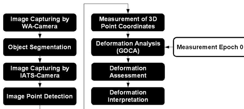
Figure 3 - Developed measurement procedure.
