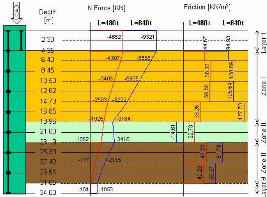
Figure 5: Sensor topology and results obtained by monitoring during the axial compression test
