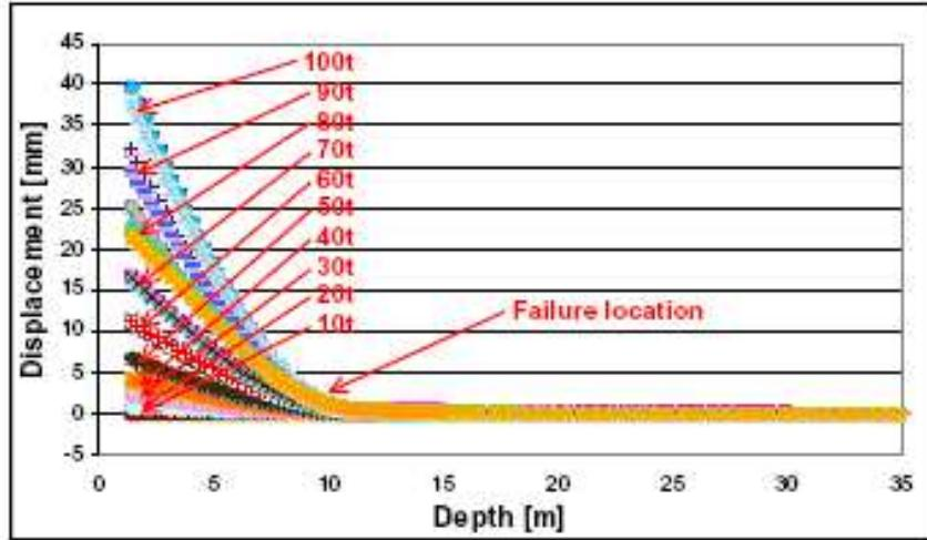
Figure 6: Deformed shapes of the pile and identification of failure location
