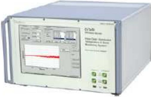
Figure 3: DiTeSt Reading Unit
