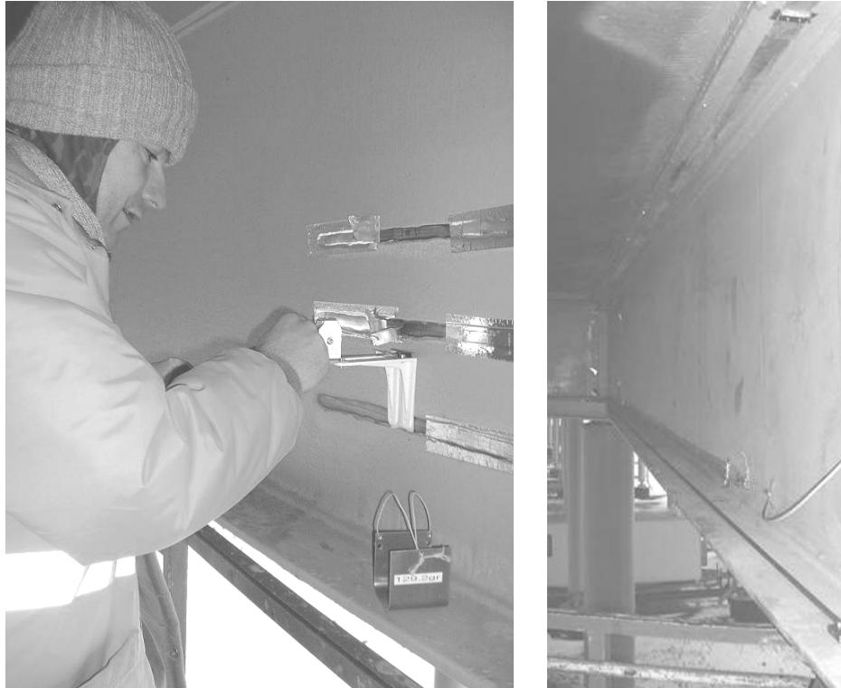
Figure 10: On-site test of SMARTape gluing procedure (left) and installed SMARTapes for full performance tests (right).
