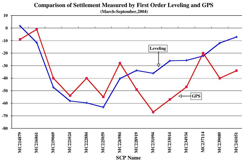
Figure 4 - Vertical deformation of survey points on the viaduct, C270 interval (1).
