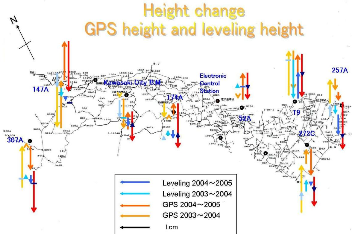
Figure 2: Successive results of comparison with respect to height change of GPS orthometric height and precise leveling orthometric height during the period 2003-2007. Electronic control station is fixed.
