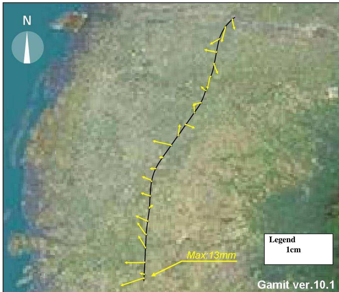
Figure 6(a): Horizontal movement of survey points on the viaduct, C270.
