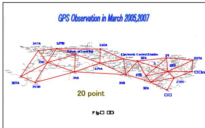
Figure 1- Occupied stations for GPS/leveling work during The period from 2003 to 2007 respectively
