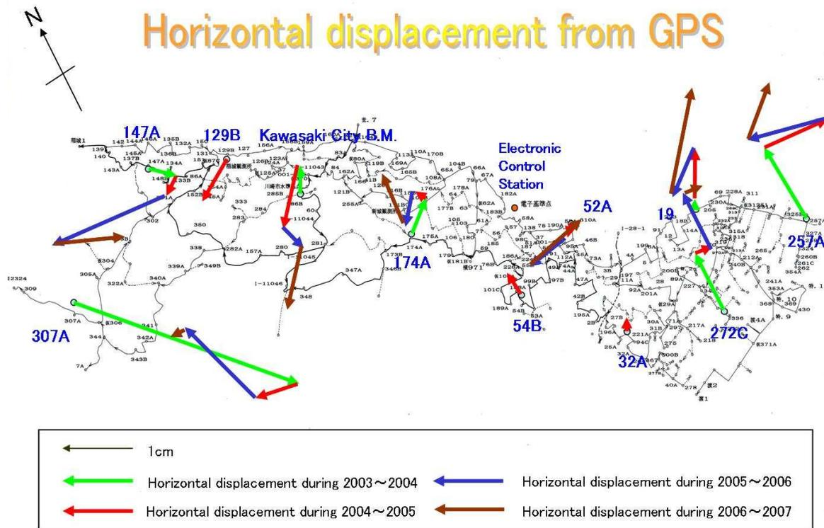
Figure 3: Successive displacement vector in Kawasaki from 2003 to 2004, from 2004 to 2005, from 2005 to 2006, and from 2006 to 2007.
