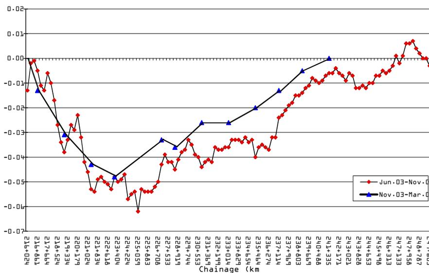
Figure 5: Vertical deformation of survey points on the viaduct, C270 interval (2).
