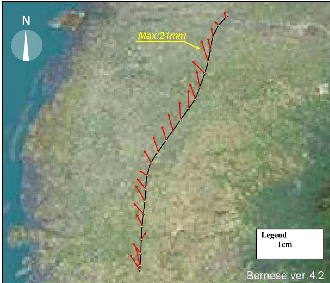
Figure 6 (b): Horizontal movement of survey points on the viaduct, C270.
