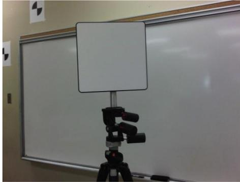
Figure 6: Spectralon target mounted on a camera tripod with a tri-axis rotation head
