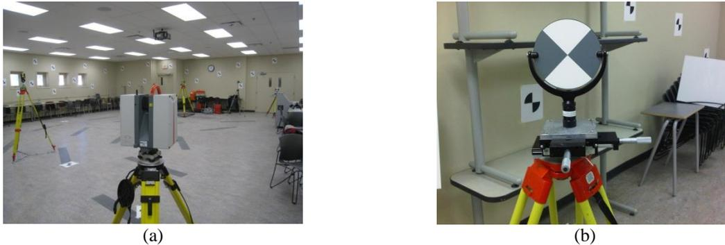
Figure 4: a) Room used for the deformation analysis experiments. b) Signalized target mounted on a translation stage
