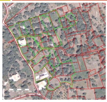
Cadastral survey produced by the contractor (in red) cadastral survey produced by KT (in green) Two cadastral units in a rural area on a Greek island that have suffered long and multiple failures of the traditional procedures.
