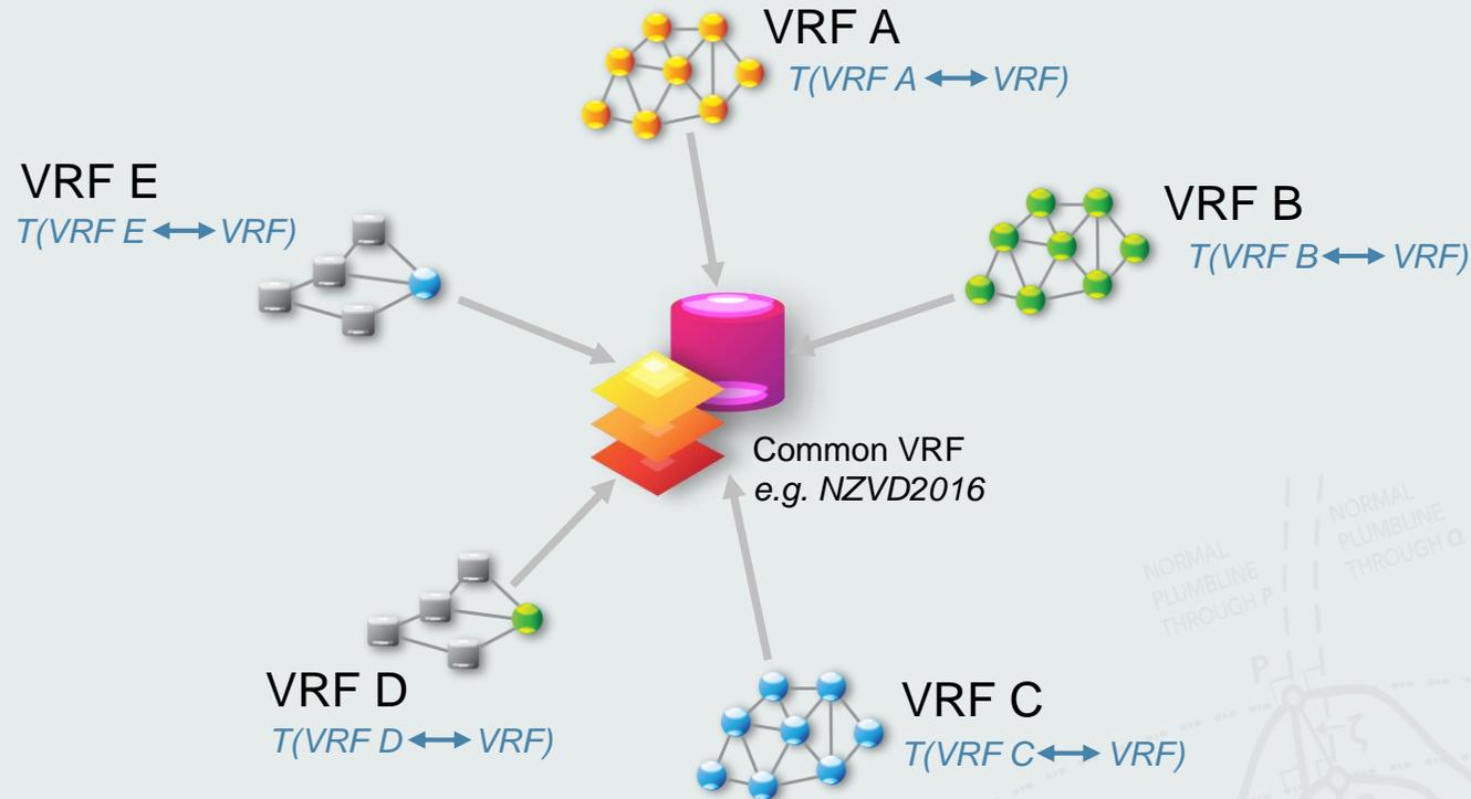
Registering GIS datasets to a common VRF can be accomplished using **vertical transformations**.
