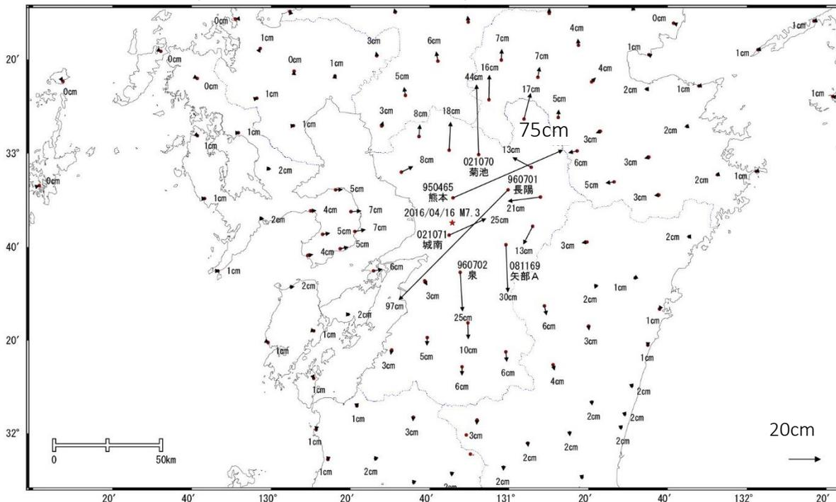
Displacement detected by ALOS-2 InSAR
