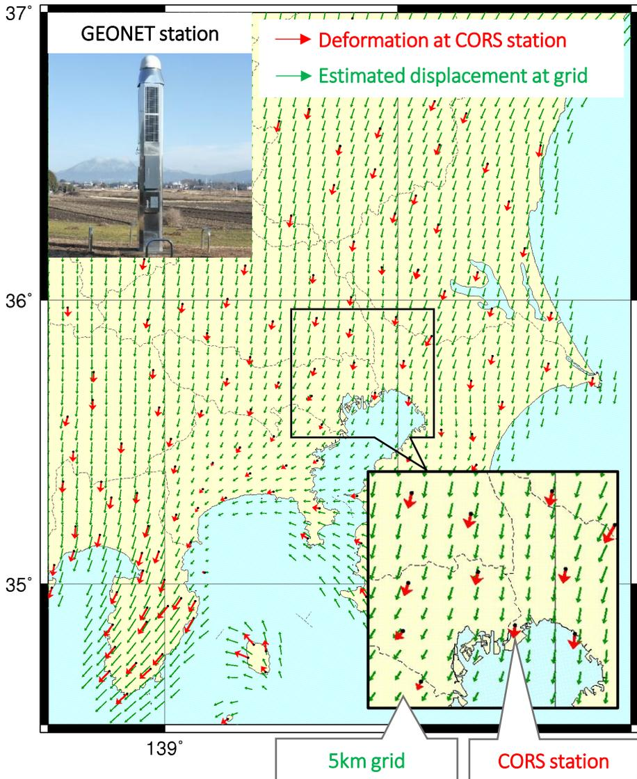
1) Cumulative crustal deformation is calculated from coordinate time series at each CORS station (average spacing 20km)
