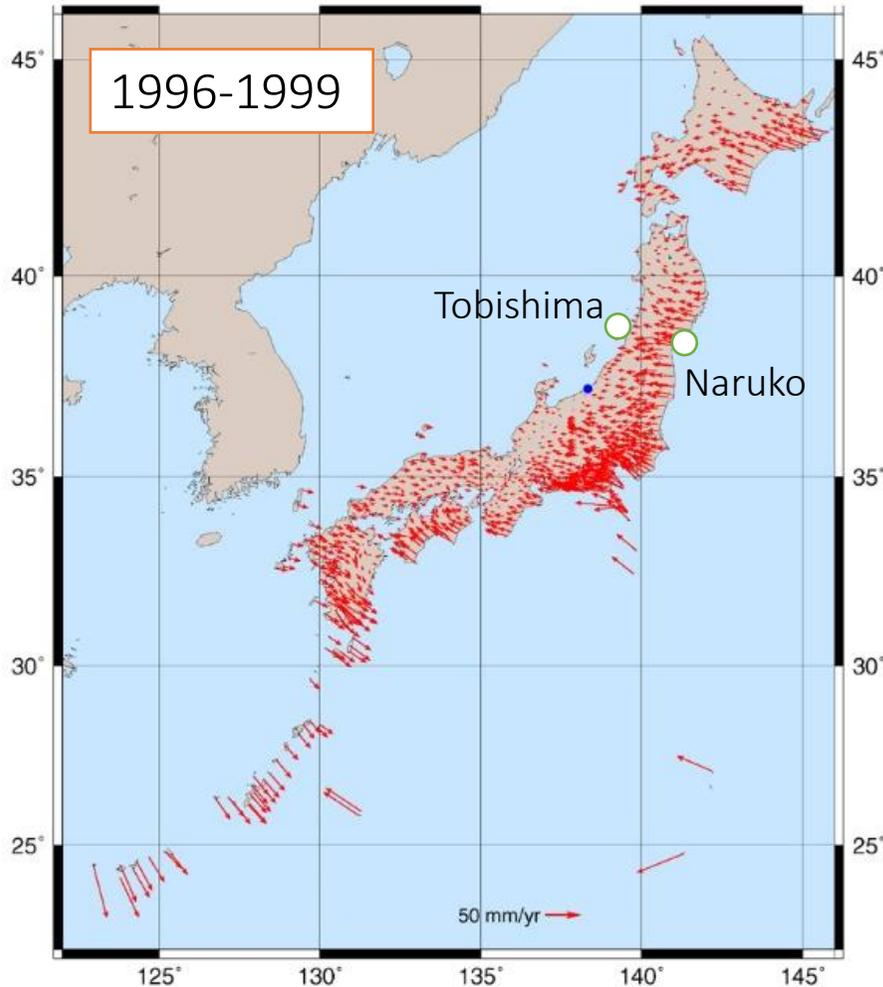
Horizontal displacement vector map detected by GEONET coordinate time series
