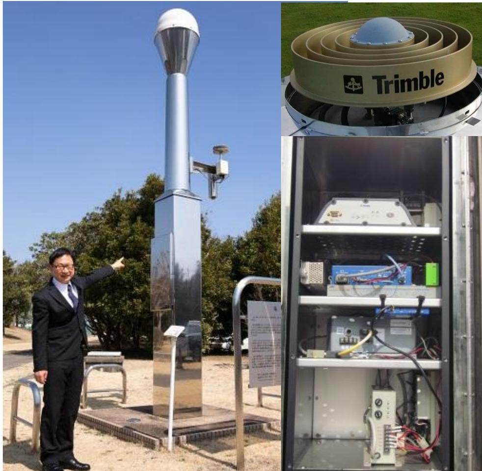
GEONET station “Tsukuba” at GSI headquarters and an antenna and equipment
