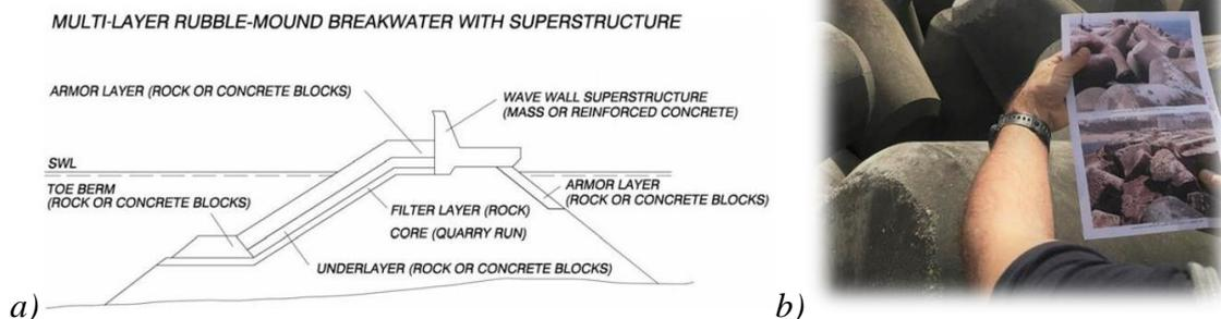
*Fig. 1: a) A typical RMB with superstructure; b) Visual inspection (comparison of photos) in a point of section B of Ericeira's breakwater.*
