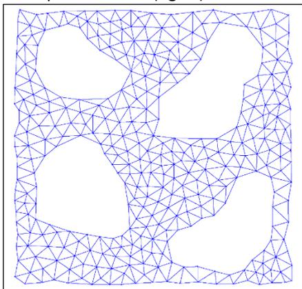
Figure 7a. Delaunay Triangulation using breaklines
