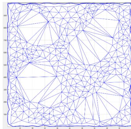
Figure 7b. Delaunay Triangulation without using breaklines
