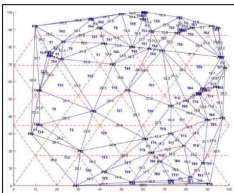
Figure 1. Comparison of vertices of a TIN vs equilateral triangle grid
