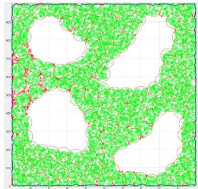
Figure 4b. Sensor deployment for medium density, R=40m and N=183
