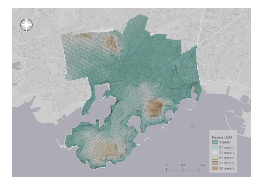
Digital Elevation Model Source: Eurostat (Copernicus) Sp. Resolution: 10m Vertical accuracy of 2.9m
