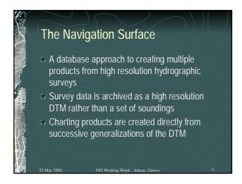
The adoption of a DTM as the hydrographic survey product and the archived survey database has significant implications for hydrographic practice and the nautical charting process
