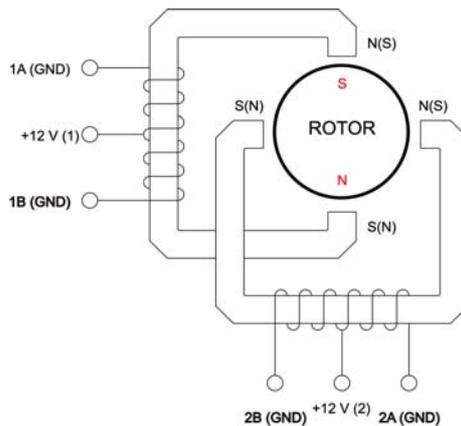
**Fig. 4.** Unipolar stepper motor schema.
