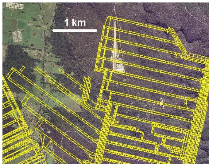
**Figure 2.** The aerial photography of the test site overlaid with the underground longwall mining plan (yellow lines).
