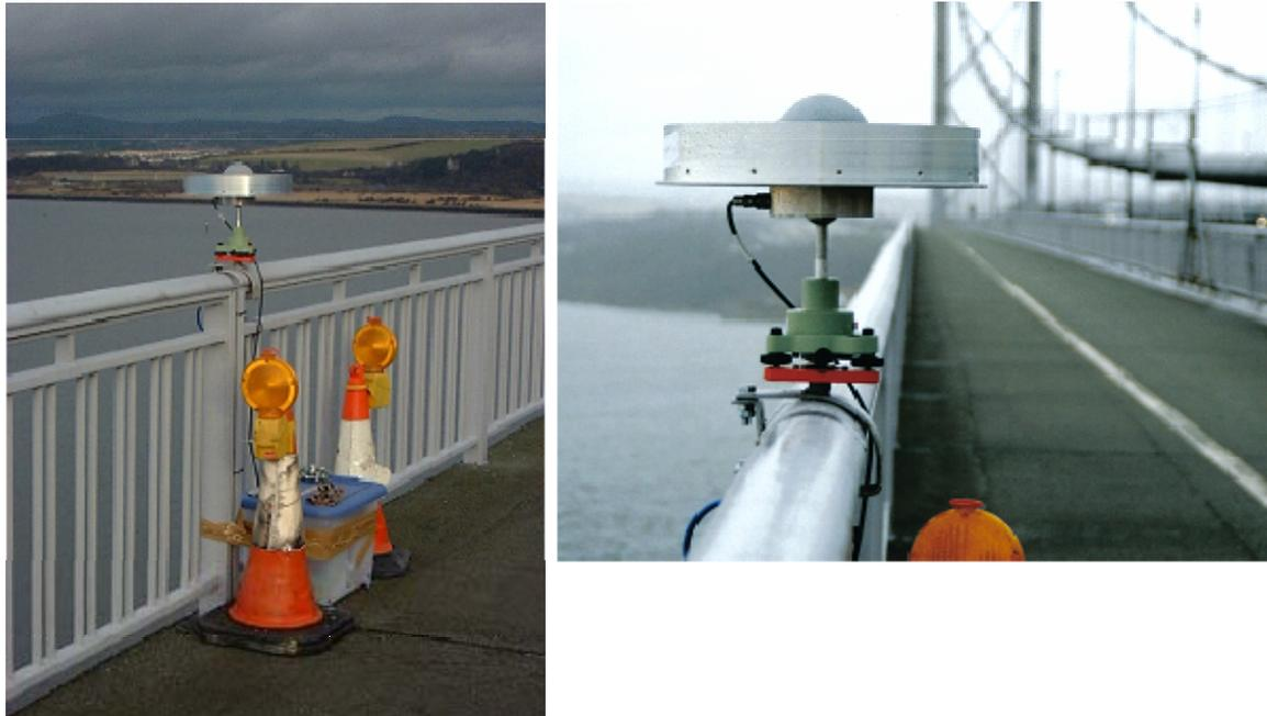
**Figure 3.** A GPS receiver located on the bridge.
