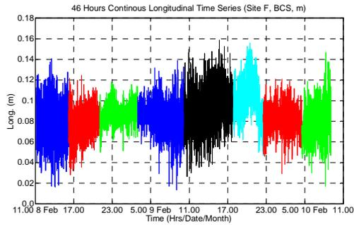
**Figure 5.** Longitudinal Deflections of Bridge site F over the 46 hour trial (Bridge Coordinate System).
