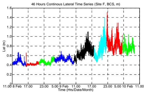
**Figure 6.** Lateral Deflections of Bridge site F over the 46 hour trial (Bridge Coordinate System).
