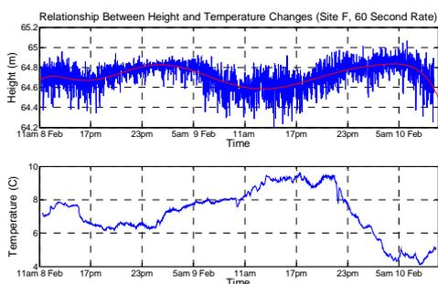
**Figure 8.** Relationship between air temperature and height location of the Bridge Deck at site F.
