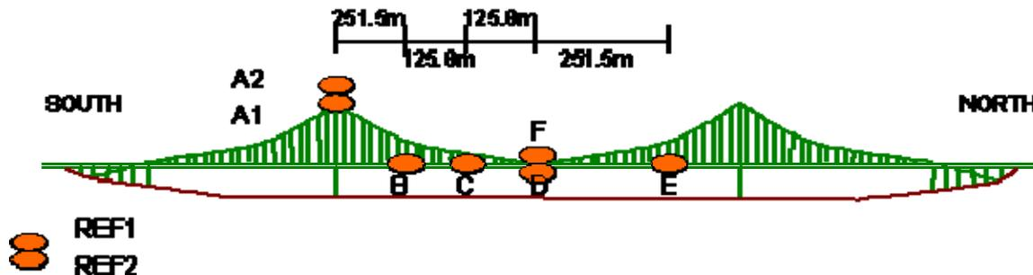
**Figure 1.** The GPS receiver locations on the Forth Road Bridge.
