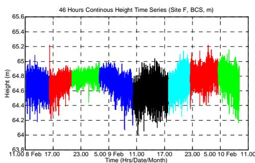
**Figure 4.** Height Deflections of Bridge site F over the 46 hour trial (Bridge Coordinate System).
