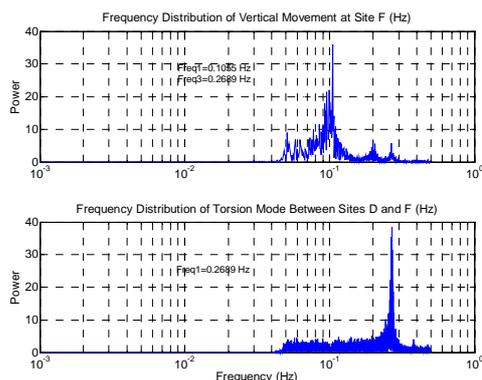
**Figure 7.** Natural Frequencies and Torsional Frequency of the Bridge.
