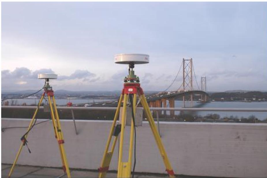
**Figure 2.** Two Leica AT503 Choke Ring antennas located adjacent to the Forth Road Bridge.
