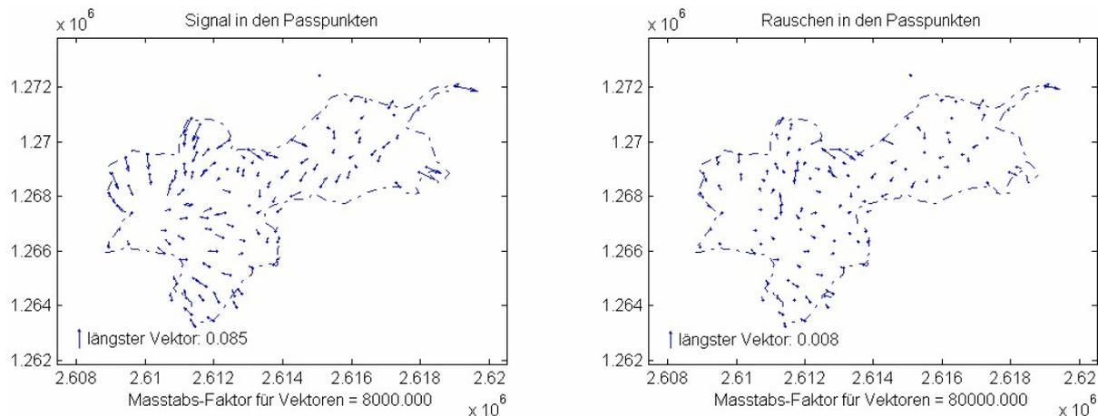
**Figure 8.** Canton of Basel-Stadt, transformation LV03 → LV95. Left: Signal estimate, right: noise estimate scaled by a factor of 10. Note that the noise varies randomly. Length unit [m].
