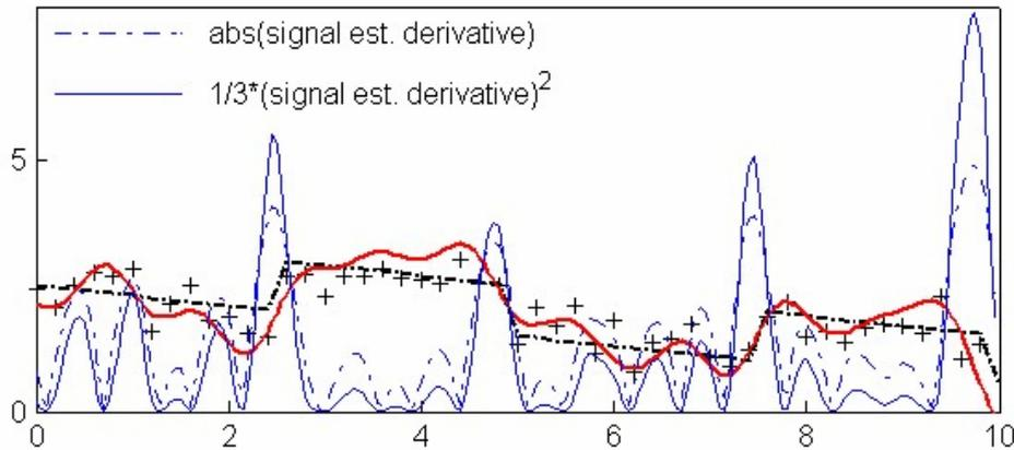
**Figure 7.** Detection of signal flows using the signal derivative of the GCV estimation. The derivative shows high peaks at the boundaries of the four signal flows, which thus can be detected.
