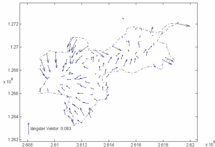
**Figure 1.** Canton of Basel-Stadt: Adjustments of LV03-coordinates of estimated Helmert transformation LV03 ↔ LV95 based on 114 fiducial points. Length unit [m].
