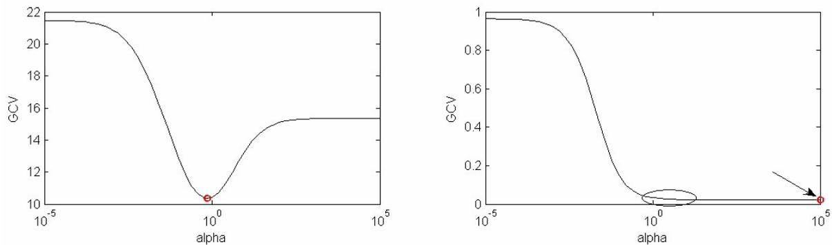
**Figure 6:** Left: A well defined minimum of  $GCV(\alpha)$ . Right:  $GCV(\alpha)$  with badly defined minimum marked by the arrow. Then  $\alpha$  has to be chosen manually in the region marked by an oval, where  $GCV$  reaches practically its minimum.
