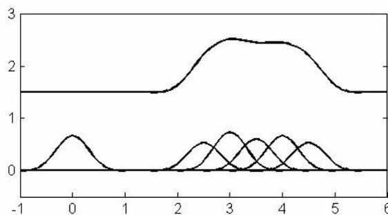
**Figure 2.** Left below: A B-spline basis function  $b(t)$ , right below: shifted and scaled B-Spline basis functions  $k_i/\alpha \cdot b(t-t_i)$ ,  $i=1, \dots, 5$ , above: sum  $1.5 + \sum k_i/\alpha \cdot b(t-t_i)$ , 1.5 is added only for the clarity of the figure.
