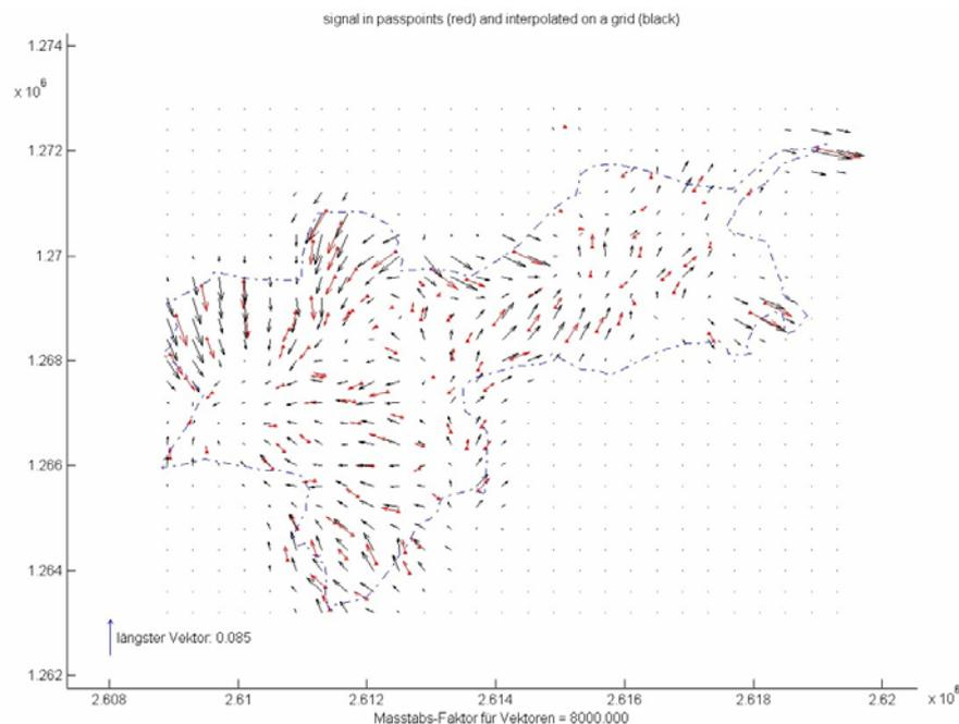
**Figure 9.** Canton of Basel-Stadt, transformation LV03 → LV95. Signal estimate on fiducial points (red) and its interpolation on a grid (black). Length unit [m].
