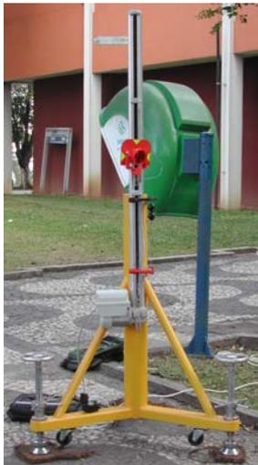
**Fig. 1** - The oscillator 2D and the standard prism positioned on the industrial pillar
