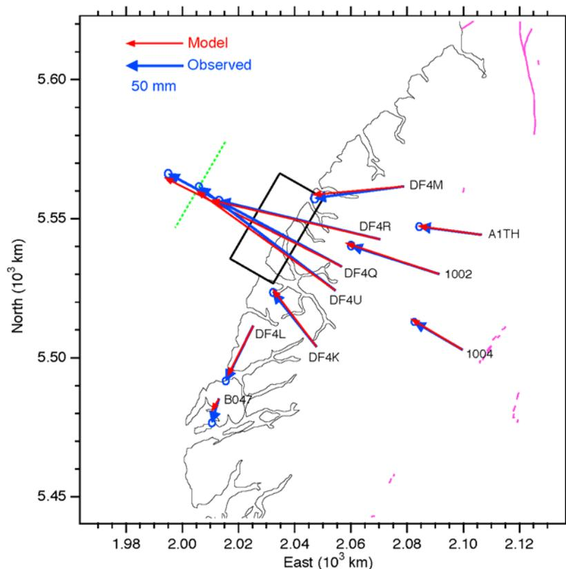
**Figure 3:** A comparison of the predicted displacements (red arrows) computed using the dislocation model (Beavan and Wallace 2004); and the observed displacements (blue arrows) based on the GPS calculated displacements. The projected fault is represented by the green dashed line and the slip surface is represented by the solid black rectangle.
