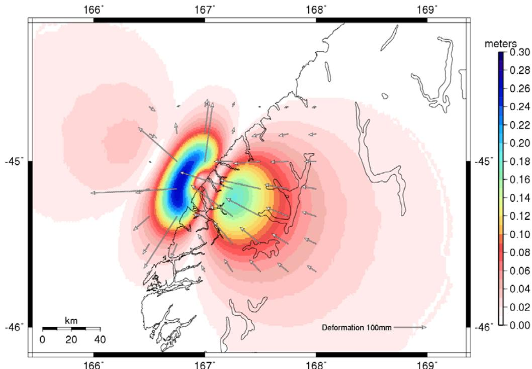
**Figure 4:** Contour and direction plot of the Fiordland deformation model. Contours are spaced at 0.01m intervals. The scale bar indicates the magnitude of the deformation represented by each colour.
