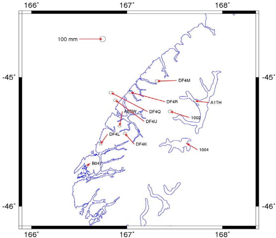
**Figure 2:** Station displacement caused by the Secretary Island earthquake, 23rd August 2003. Displacement is relative to a fixed Pacific plate. The 95% error ellipses for the displacements are shown.
