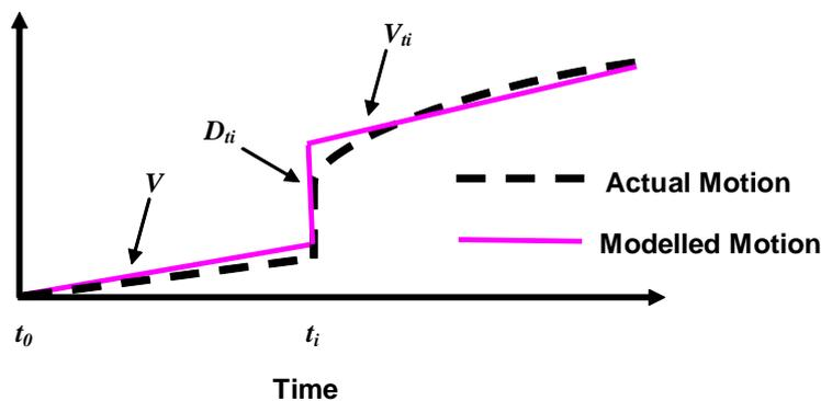
**Figure 1:** The dashed line represents the true motion and the solid line (pink) represents the modelled motion as described by the NDM. The velocity before and after  $t_i$  may not be the same. The event displacement is  $D_{ii}$ .
