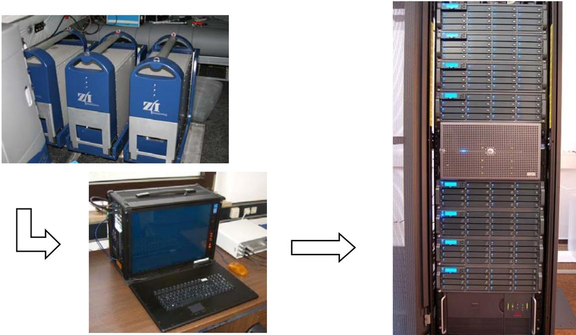
**Figure 2:** Data flow from flight data storage system via copy station to image server
