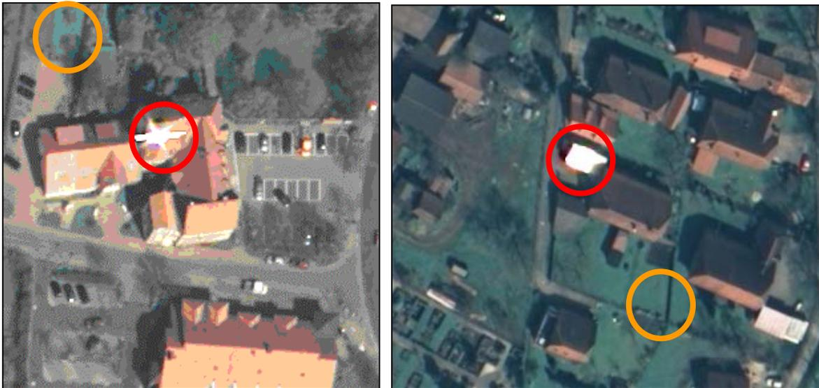
**Figure 5:** Radiometric effects of total reflection (red circles) and influence of the near infrared on the blue channel (orange circles), flight for Land Survey Department Lower Saxony
