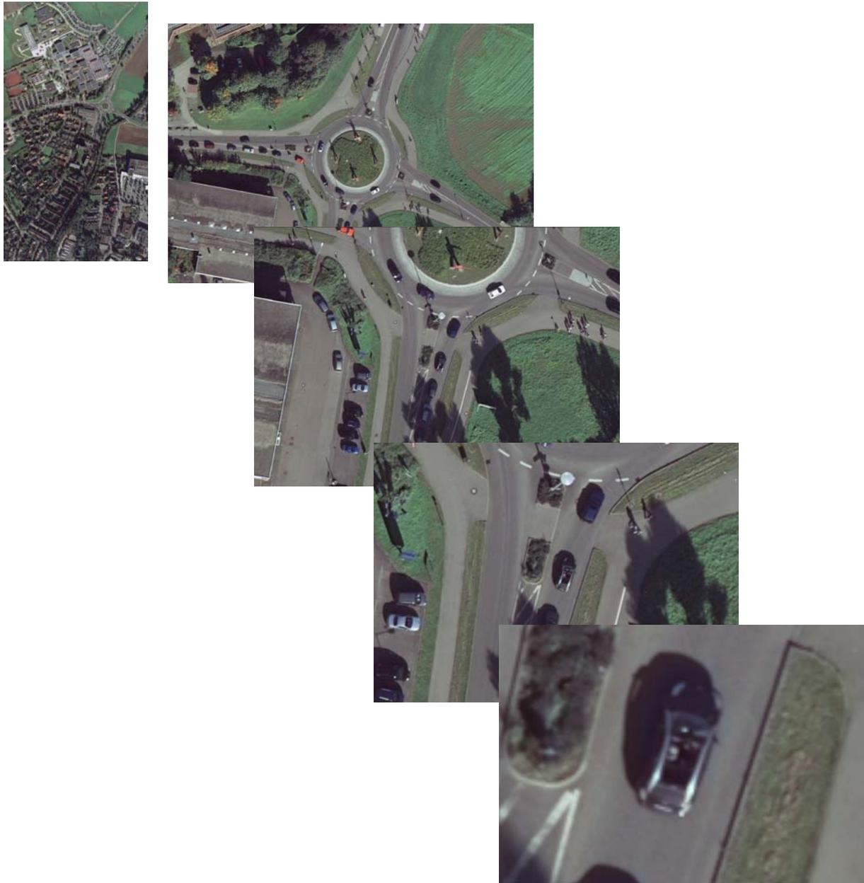
**Figure 10:** Enlargement of color image with GSD = 0,06 m (original at the upper left corner)
