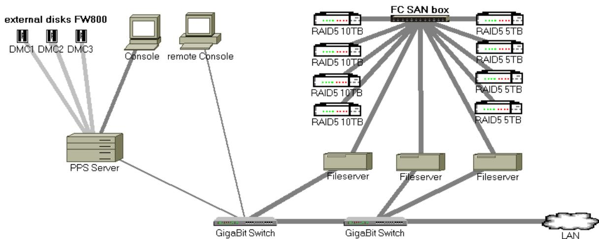
**Figure 3:** Processing and storage network of DMC post processing
