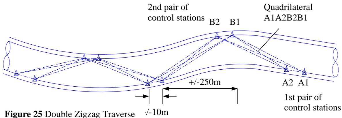
**Figure 25** Double Zigzag Traverse
