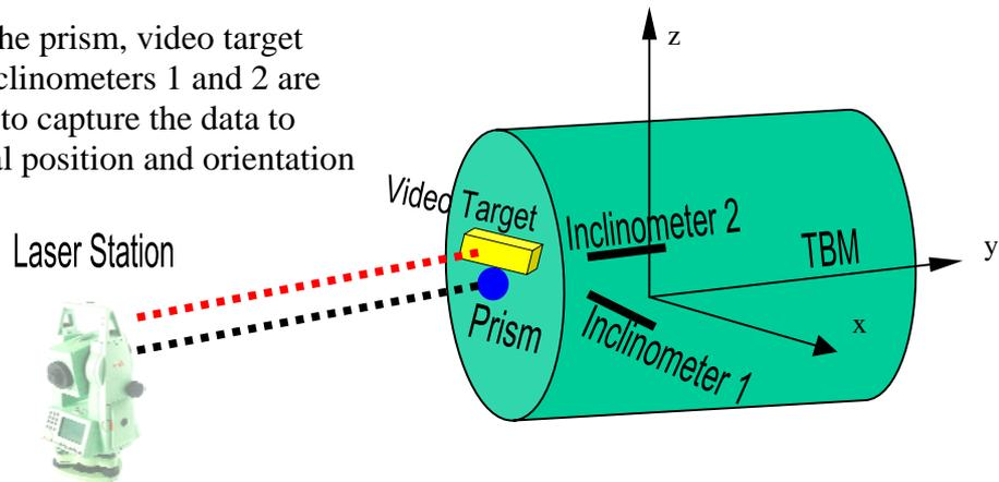
**Figure 15** The mechanism of data acquisition of the tunnel guidance system
