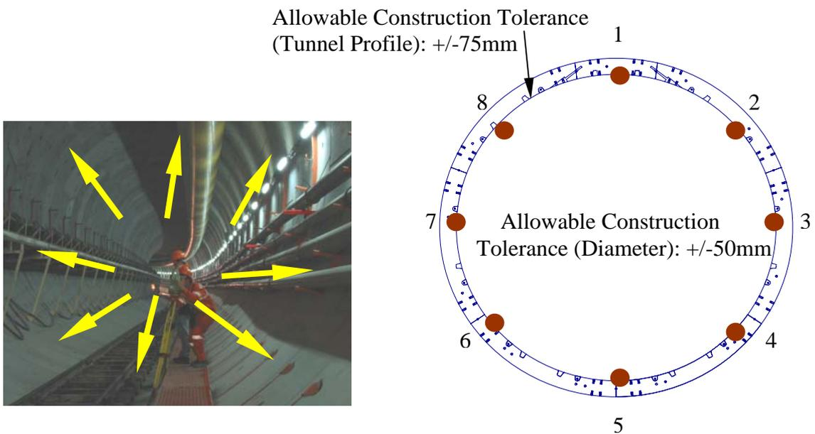
Figure 22 A standard eight point wriggle survey
