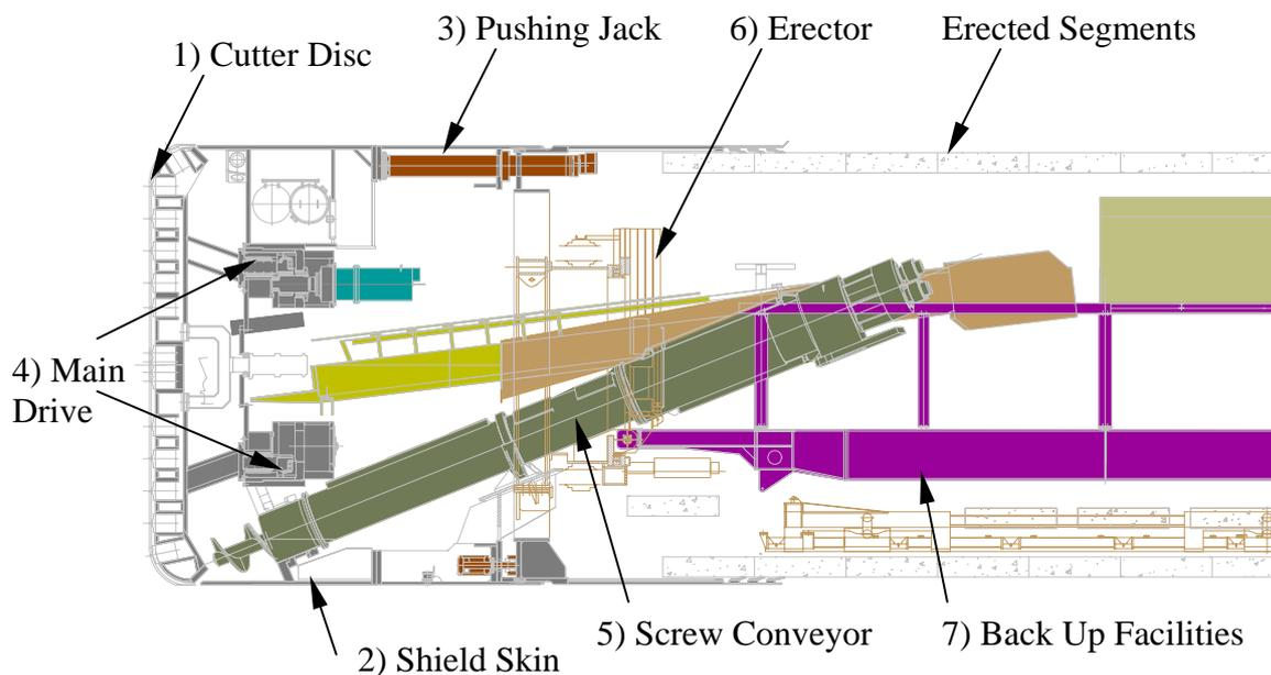
**Figure 1** Typical Layout of a TBM
