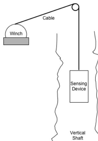
**Figure 1:** Vertical shaft inspection concept
