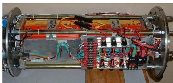
**Figure 10:** Pod primary batteries and power controller
