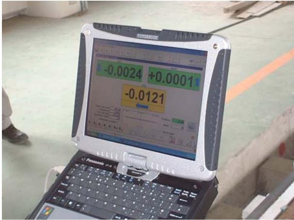
**Fig.3.15** Real Time Comparison between Coordinates of Station Survey and Design Lineshape for Adjustment.
