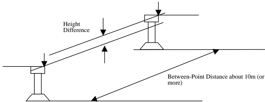
**Fig.3.3** Elevation Survey
