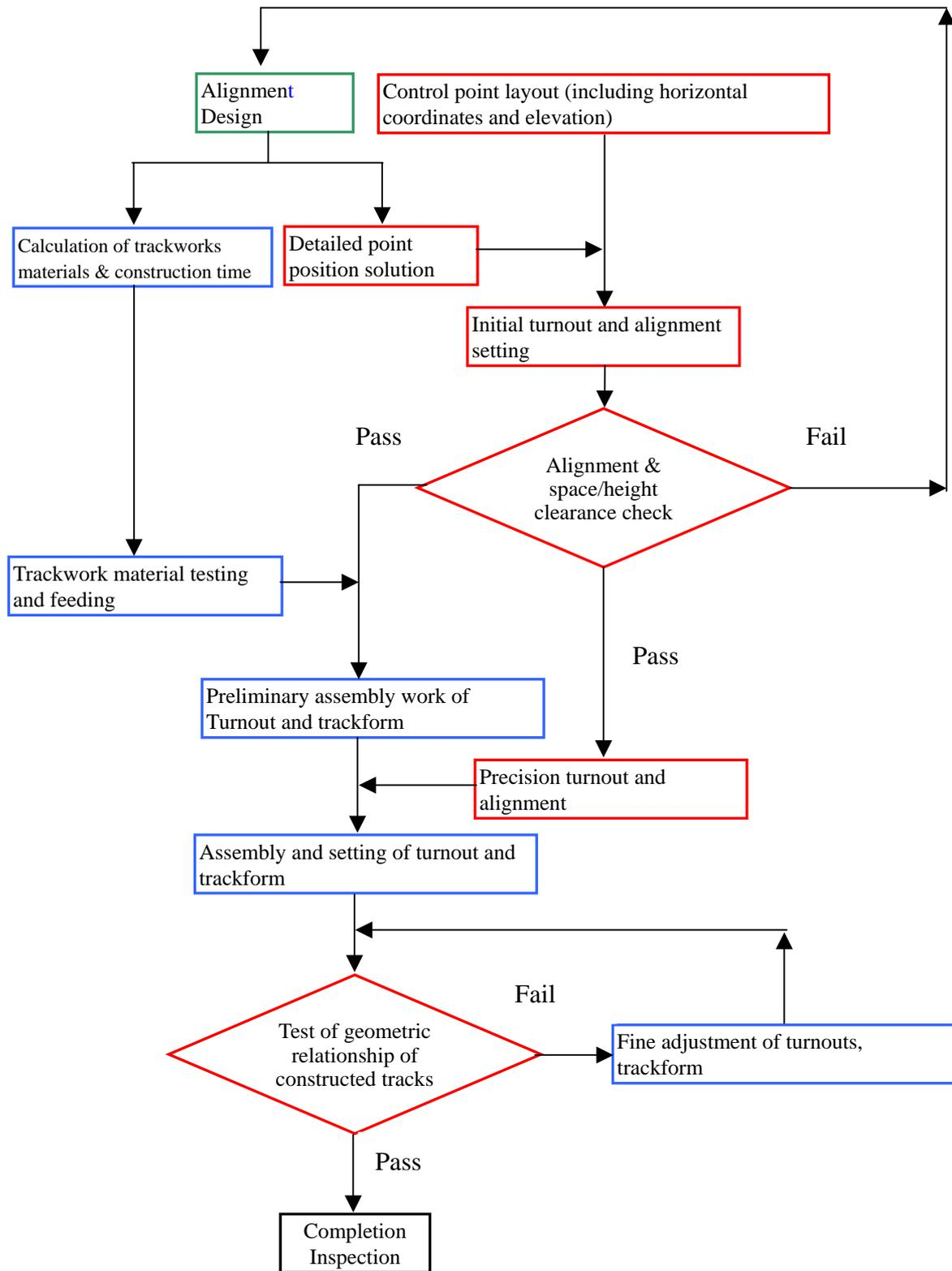
**Fig.2.1** Relations of Trackworks Construction and Survey Operations
