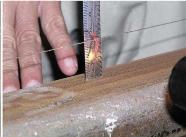
**Fig.3.8** Conventional Positioning Elevation Survey Method
