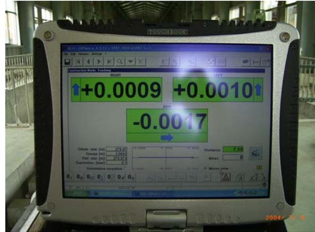
**Fig.3.16** Post-Adjustment Measurement. Difference from design is less than 2mm. Green indicates pass; yellow indicates over.
