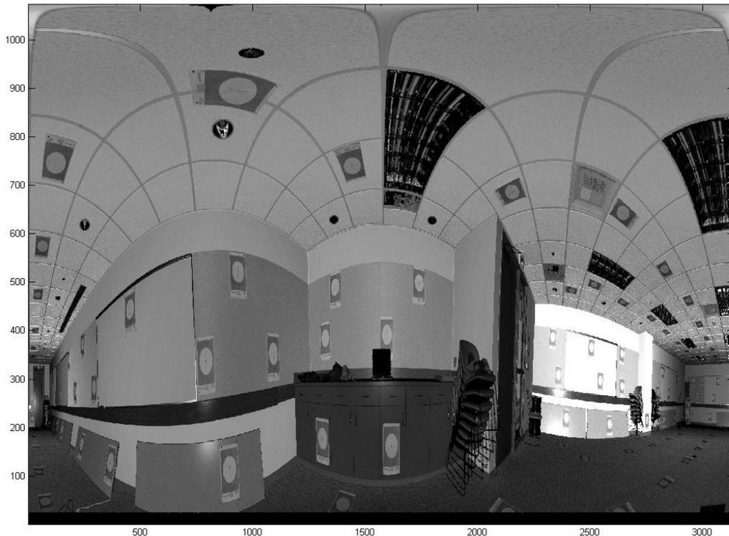
**Figure 5.** Two-dimensional point cloud view for target measurement.
